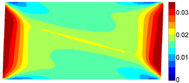
Figure 6.18: FEM simulation of simple shear test, colorbar in radian
