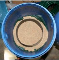
Experimental set-up of the wood ash leaching Fig. 2: Ring for water distribution 1: Fig. experiment in barrels
