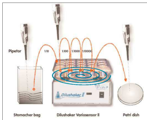
Figure 30: Principle of the dilution step procedure by use of the Dilushaker system (IMAGE 9, 2011)
