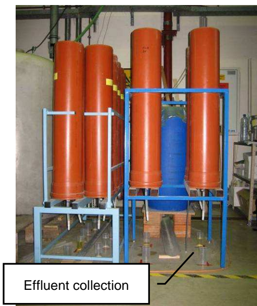
Figure 3.3-9: Columns; cups for effluent collection
