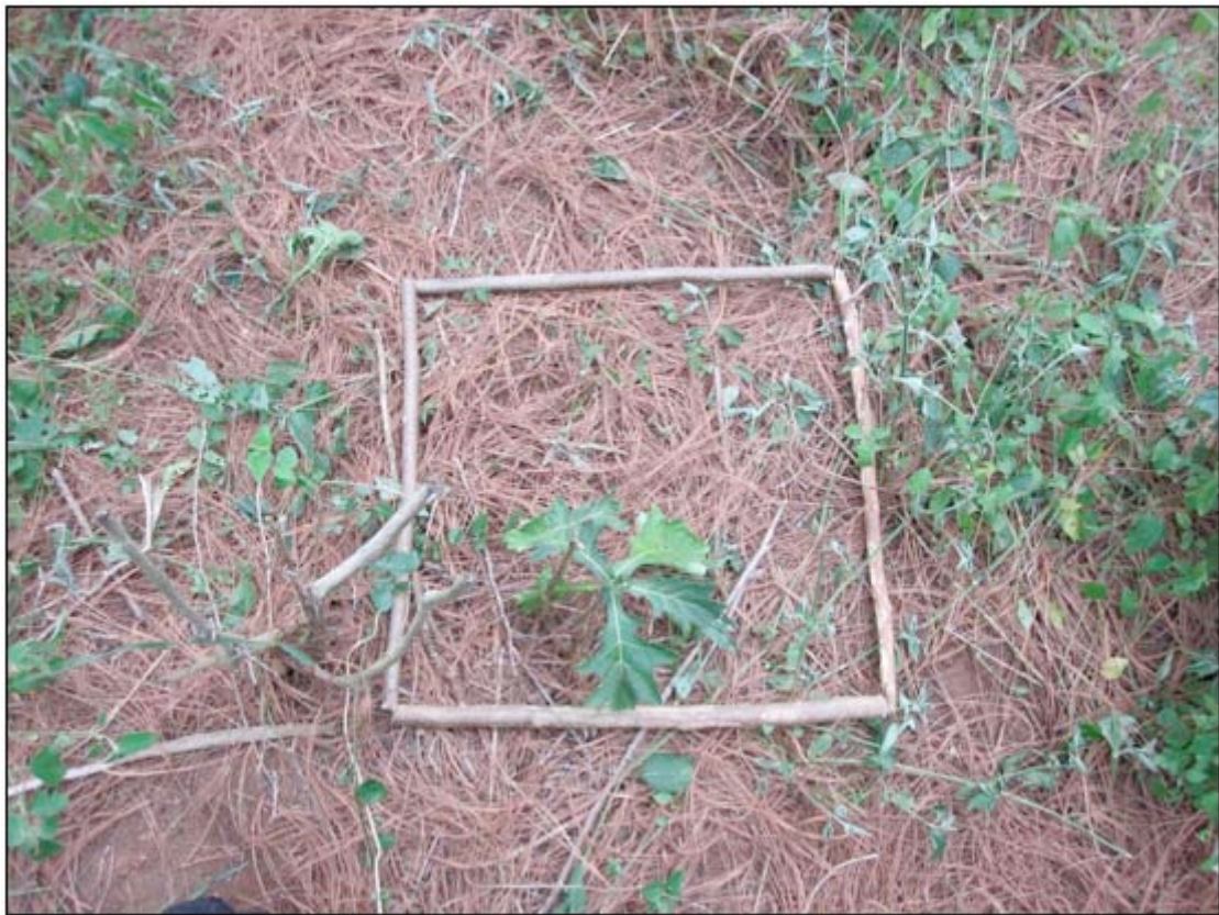
Figure 15: Example of 50x50 cm frame used for collection of litter layer.
