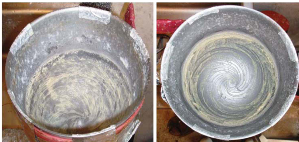
Figure 2 Deposits from sizing agents. Left: from ASA, right: from MSOHO.
