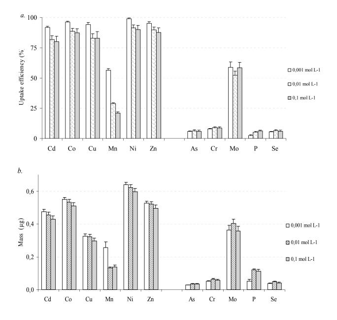
Figure 5.4.1. a) Uptake efficiency of La-Chelex 2 r esin gel; b) measured mass on the L a-Chelex 2 resin gel disc after deployment in the experimental solution containin g cationic and anionic analytes. The La concentrations used for impregnating Chelex gels were 0.1, 0.01 and 0.001 mol  $L^{-1}$ . Deployment time was 5h. Error bars represent the standard errors.
