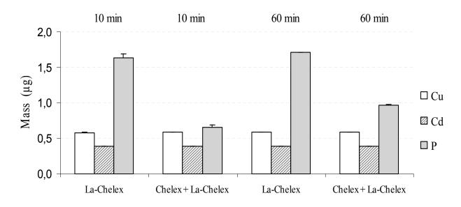
Figure 5.1.2. Measured mass of the elements on the La-Chelex and Chelex+La-Chele x resin after deployment in the experimental solution. Deployment times were 10 min and 60 min. Error bars represent the standard errors.
