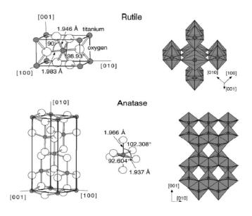
Figure 3.4.2. Bulk structures of rutile and anatase.
