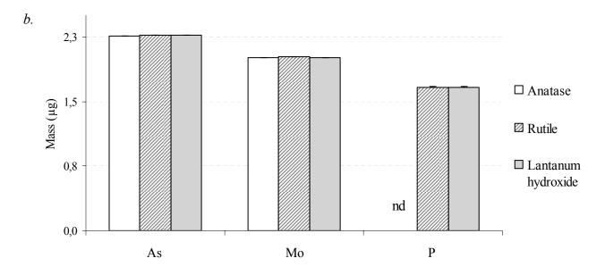
Figure 5.6.1. Uptake efficiency of different re sin gels (a) c ontaining different binding agents and measured mass on the gels (b) after deployment in the experimental solution containing cationic and anionic analytes. Anatase, rutile and lant hanumhydroxide were t ested as binding resin. Error bars represent the standard errors.
