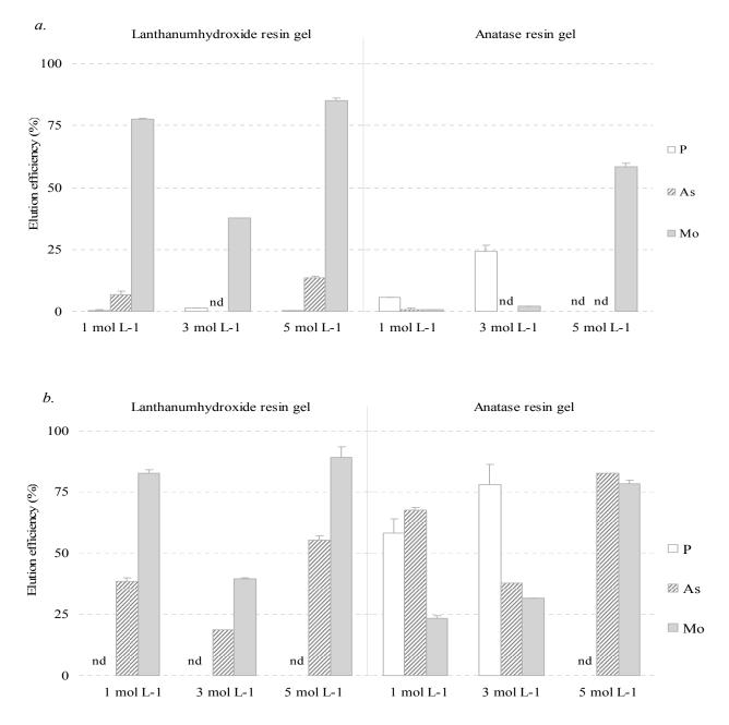
Figure 5.8.2. Elution efficiency of lanthanumhydorxide and anatase resin gels at different concentrations of HCl (a) and  $H_2SO_4$  (b). The concentrations of the acids used for elution were 1 mol  $L^{-1}$ , 3 mol  $L^{-1}$  and 5 mol  $L^{-1}$ . Error bars represent the standard errors.
