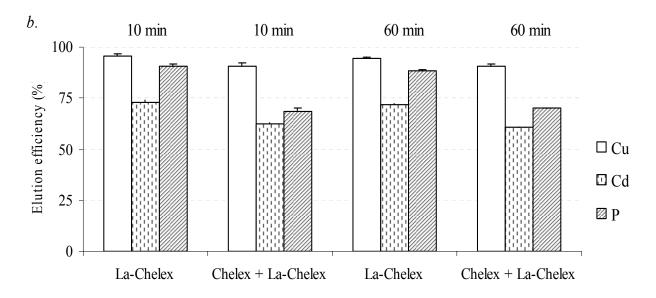
Figure 5.1.1. (a) Uptake and (b) elution efficiencies of La-Chelex and Chelex + La-Chelex (mixtu re) resins after deployment in the test solution containing cationic and anionic analytes. Deployment times were 10 min and 60 min. Error bars represent the standard errors.
