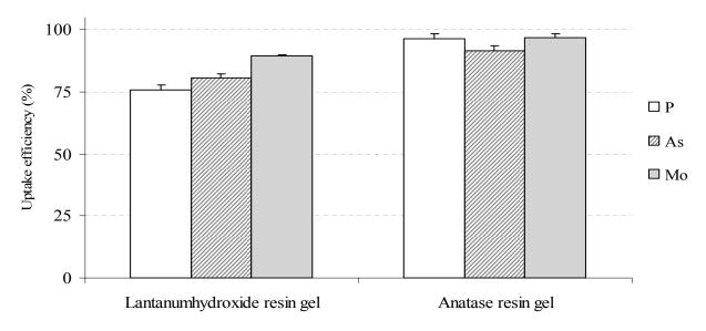
Figure 5.8.1. Uptake efficiency of lanthanumhydroxi de resin gel and anatase resin gel after deployment in the experimental solution containing anionic analytes. Error bars represent the standard errors.
