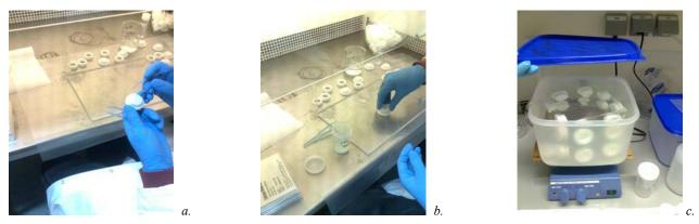
*Picture 4.5.1.: a. The base of DGT device; b. The base and top are assembled together after placing binding and diffusive layers; c. DGT devices are in application*
