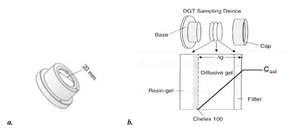
Picture 3.1.1. DGT-plastic sampling device: a. device is assembled, b.device is not assembled (Warnken et al., 2007)
