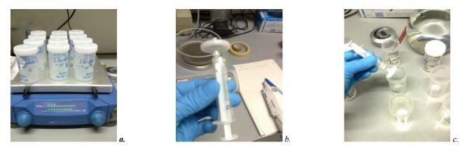
Picture 4.7.1.: a. The DGT resins gel discs were shaken during deployment; b. and c. Syringe filters were used to filter the immersion solution
