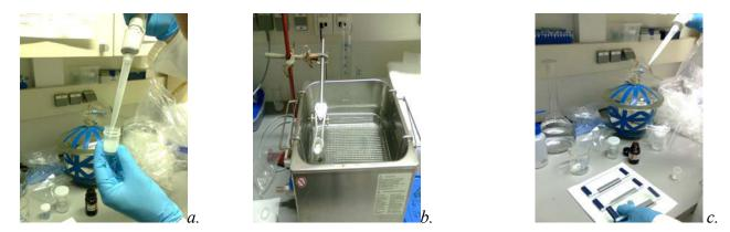
Pictures 4.2.1.: a. A pipette was used for mixing the La-Chelex resin with the viscous gel solution; b. An ultrasonic bath was used for mixing the powdery mineral resins with the viscous gel solution; c. Glass plates were used to prepare DGT resin gels.
