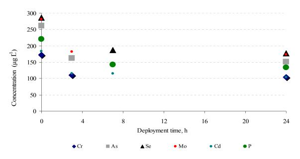
Figure 5.5.1. The concent ration of the experimenta l solution after different times of dep loyment. The values at the Y axis show the initial concentration of the solution before exposure of the DGT device.
