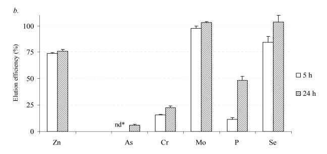
Figure 5.3.1. (a) Uptake and (b) elution efficienci es of La-Chelex 2 resin gels. Gels we re deployed in the experimental solution containing cationic and anioni c analytes. Deployment times were 5h and 24h. The acid used for elution was 1 mol L  $^{-1}$  HCl. Error bars repres ent the standard errors. Some elution efficiencies were not presented here. (nd\* - not determined).
