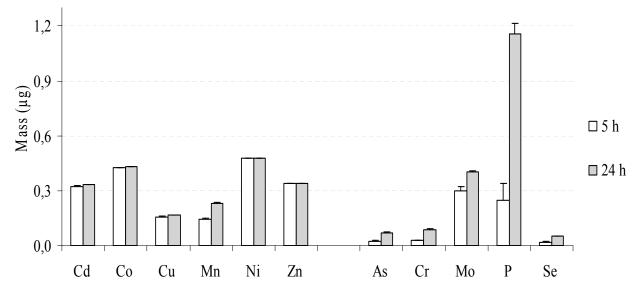
Figure 5.3.2. Measured mass of the analytes on the La-Chelex 2 resin gel disc after deployment in the test solution containing cationic and anionic analytes. Deployment times were 5h and 24h. Error b ars represent the standard errors.
