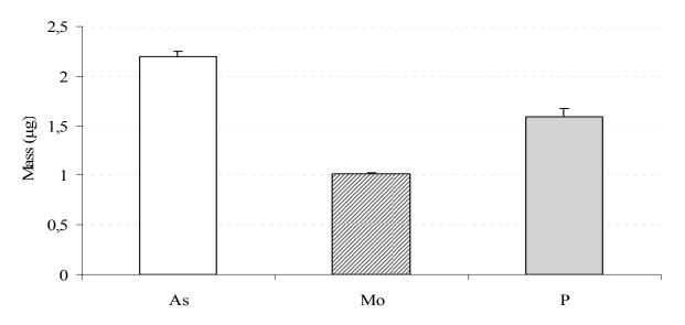
Figure 5.7.2. Measured mass of anionic analysts of lantanumhydroxide resin gel disc after deployment in the experimental solution containing anionic analytes. Error bars represent the standard errors.
