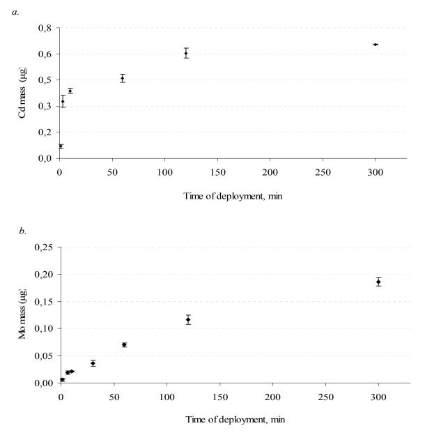
Figure 5.2.2. Kinetics of (a) cadmi um and (b) molybdenum on the L a-Chelex 1 resin gel. T he concentration in the experimental solution be fore exposure of the resin gel was 0.66  $\mu$  g mL<sup>-1</sup> for Cd and 0.50  $\mu$ g mL<sup>-1</sup> for Mo. Error bars represent the standard errors.
