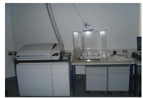
Picture 4.6.1.: a. 20 mL vials as used for the experiments; b. Sample dilution for ICP-MS analysis: c. Inductively coupled plasma mas s spectrometry (ICP-MS)
