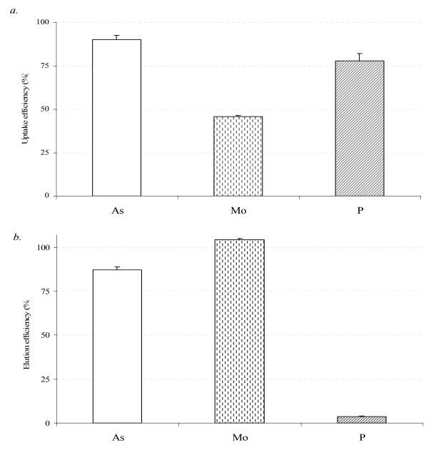
Figure 5.7.1. Uptake (a) and elution (b) efficiency of lanthanumhydroxide resin gel after deployment in the experimental solution containing anionic analytes. The eluent was 0.25 mol L<sup>-1</sup>  $H_2SO_4$ . Error bars represent the standard errors.
