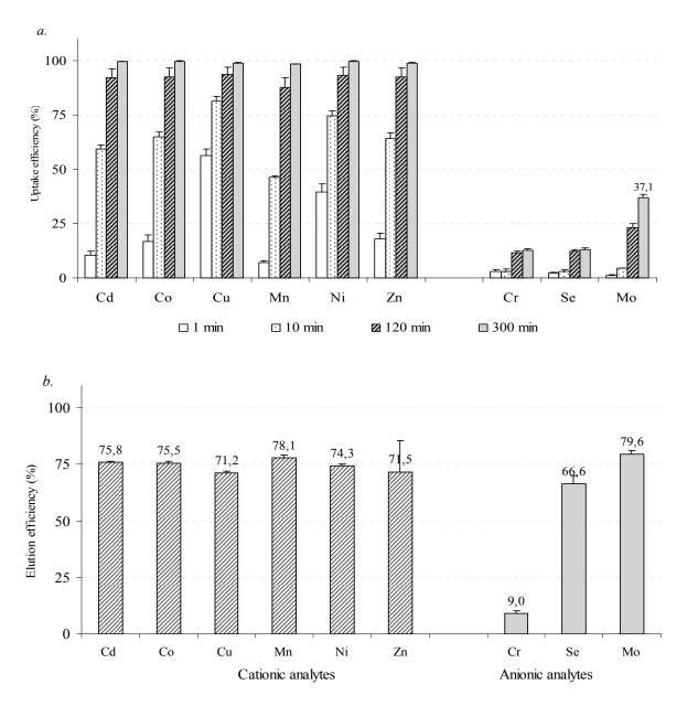
Figure 5.2.1. (a) Uptake and (b) elution efficiency of La-Chelex 1 resin gel after deployment in the experimental solution containing cationic and anio nic analytes. Deployment times were 1 min, 10 min, 120 min and 300 min. Error bars represent the standard errors.
