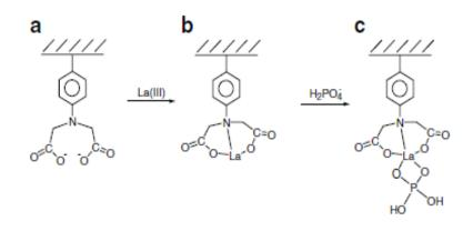
Figure 3.4.1. (a) Structure of chelex-100, (b) Chelex-100 compound with La after impregnation with La, (c) La-chelex-phosphate after deployment in phosphate solution. (After Wu et al., 2007)
