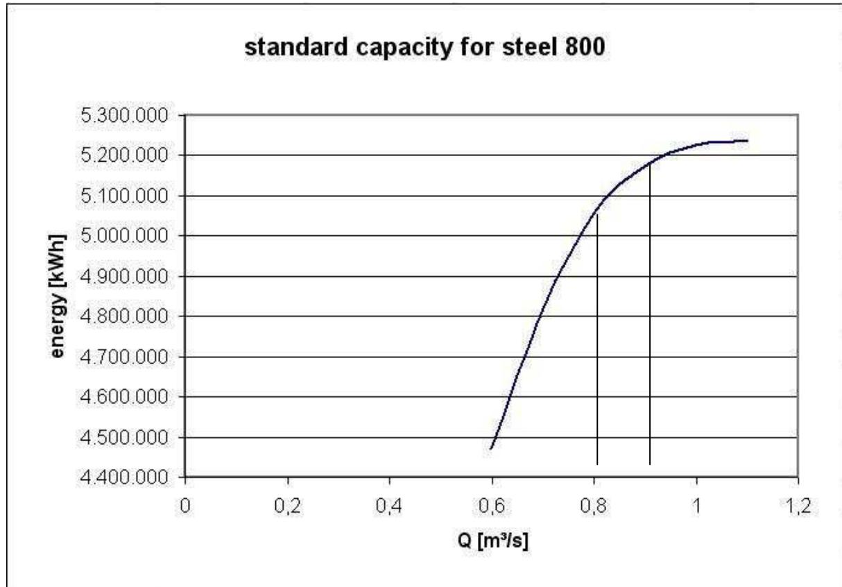
Figure 16: standard capacity for steel pipes with diameter 800 (own source)
