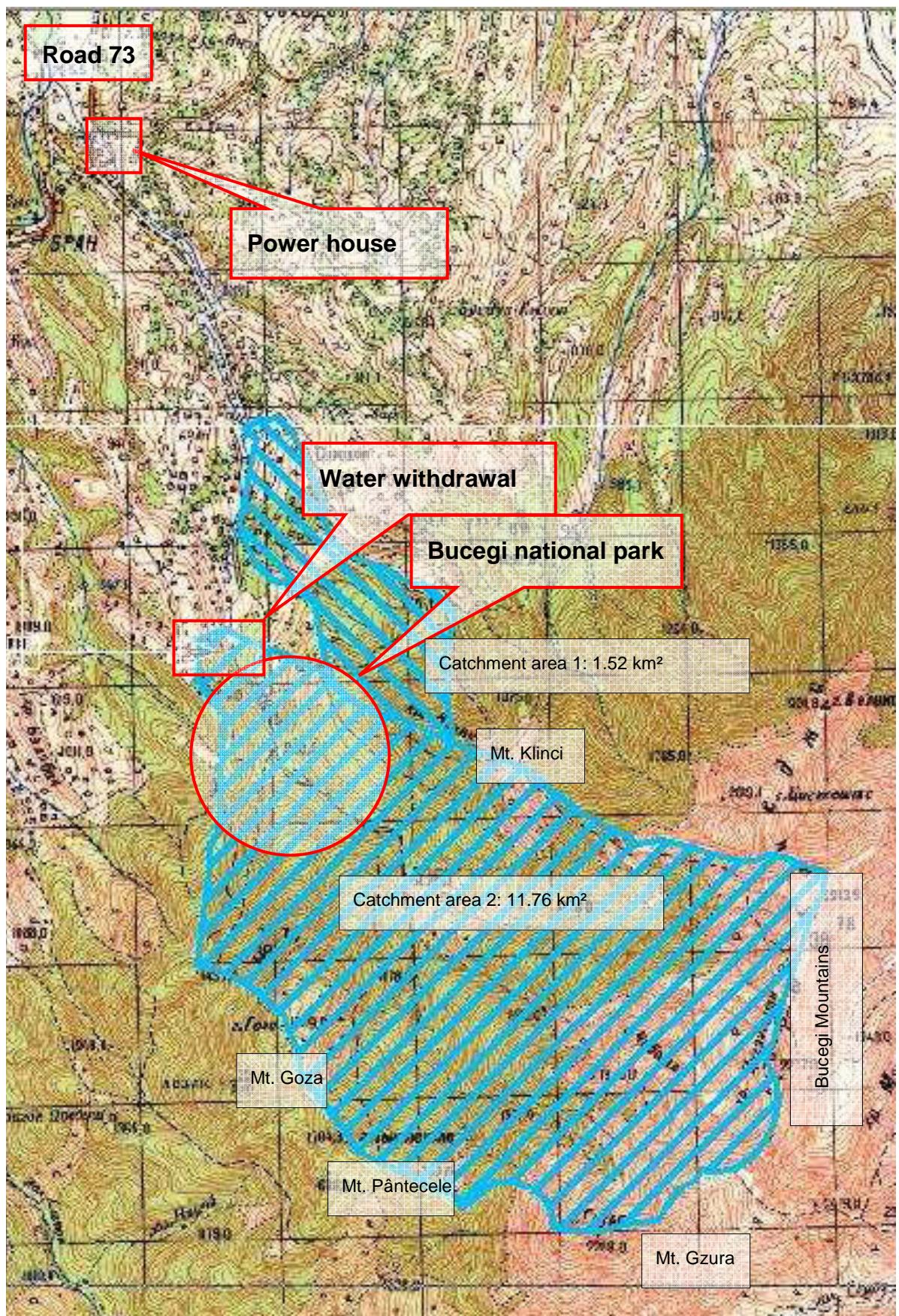
Figure 2: Catchment area and position of water withdrawal and power house (on basis of Generalhydraulics map, 1975)
