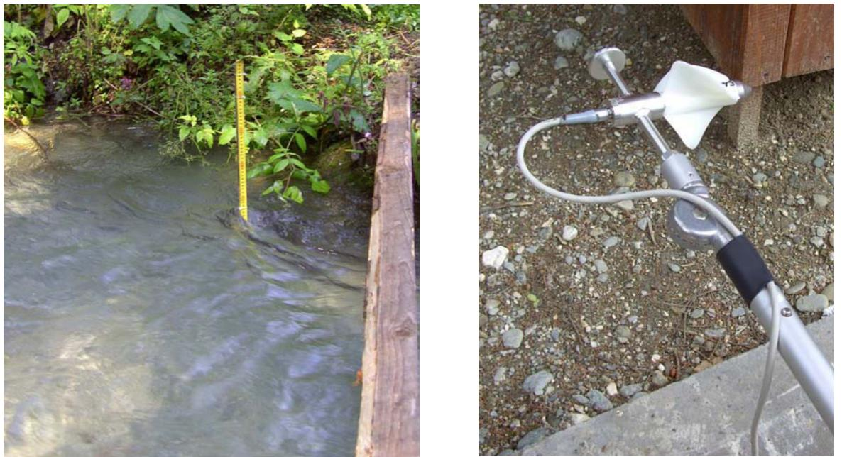
Figure 10: installed measuring device (left) and flow meter (right), (own source)
