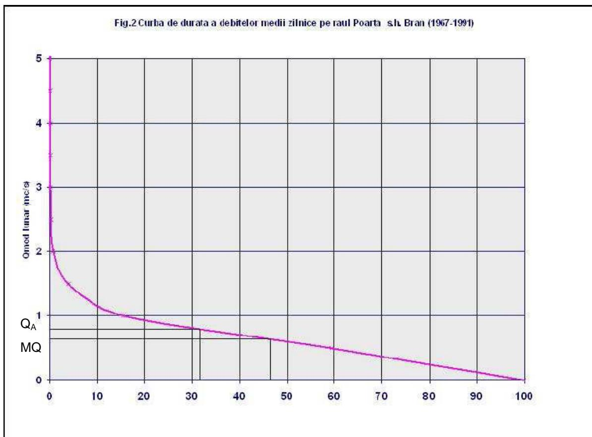
Figure 15: Duration curve of Poarta River with integrated design flow and MQ (Institutul Național de Hidrologie, 2004)
