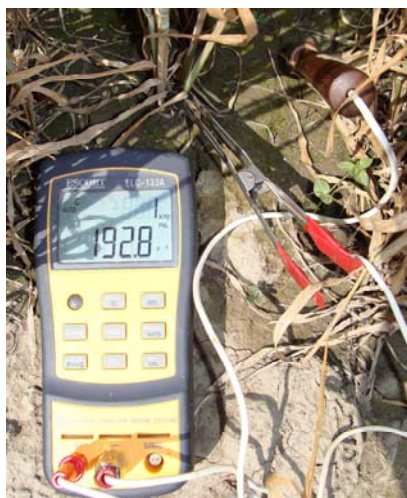
Figure 7: LCR meter the plant clamp electrode and the soil electrode
