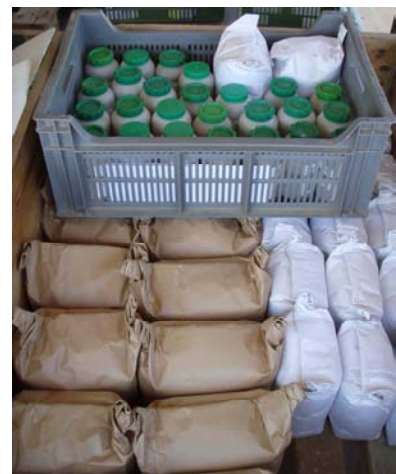
Figure 5: Samples for examining the water content (in plastic bottles) and the quality parameters (in paper bags)
