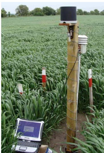
Figure 15: Local weather station for measuring precipitation, air and soil temperature and air and soil humidity
