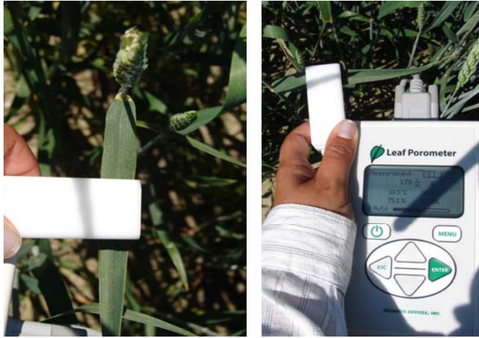
Figure 13: Leaf porometer and the application of the sensor head
