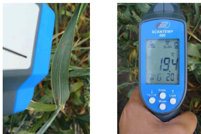
Figure 11: Infrared thermometer with the two laser points (left) and the displayed surface temperature (right)
