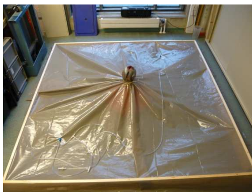
Figure 3.2: Illustration of the constructed accumulation chamber
