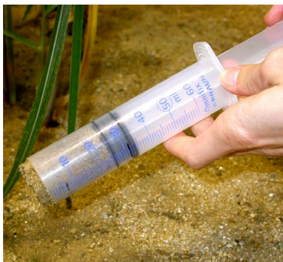
Figure 5.8: Syringe cut at the top to take samples from depths of 0-10 cm of the CW filter body
