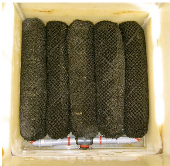
Figure 5.4: Special glass-fibre filters for the drainage layer (Plot 9 and 8)
