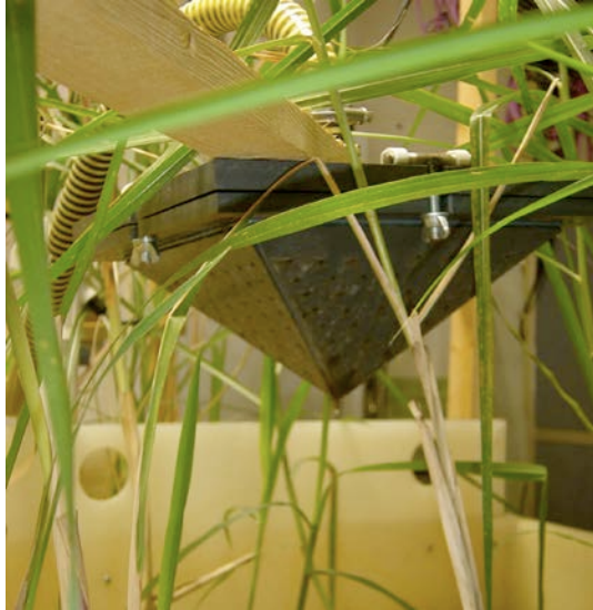
Figure 5.3: Wastewater distribution system for the PSCWs
