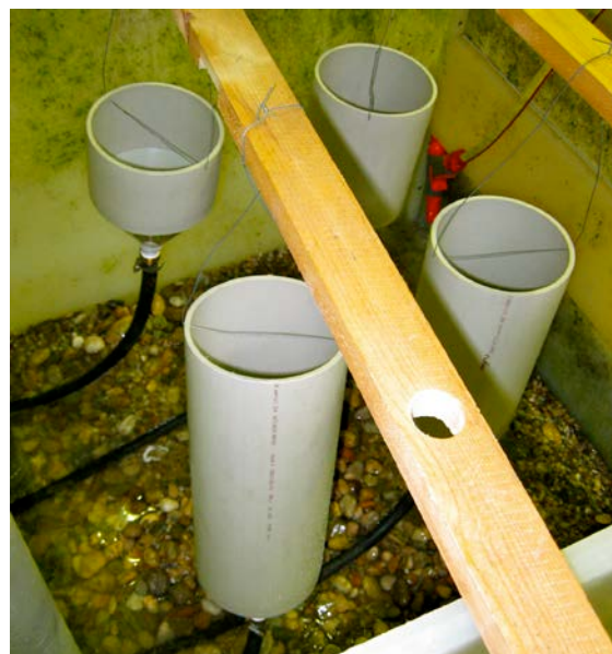
Figure 5.5: Collecting systems for the investigation for the effluents in different depths (Plot 1–5)
