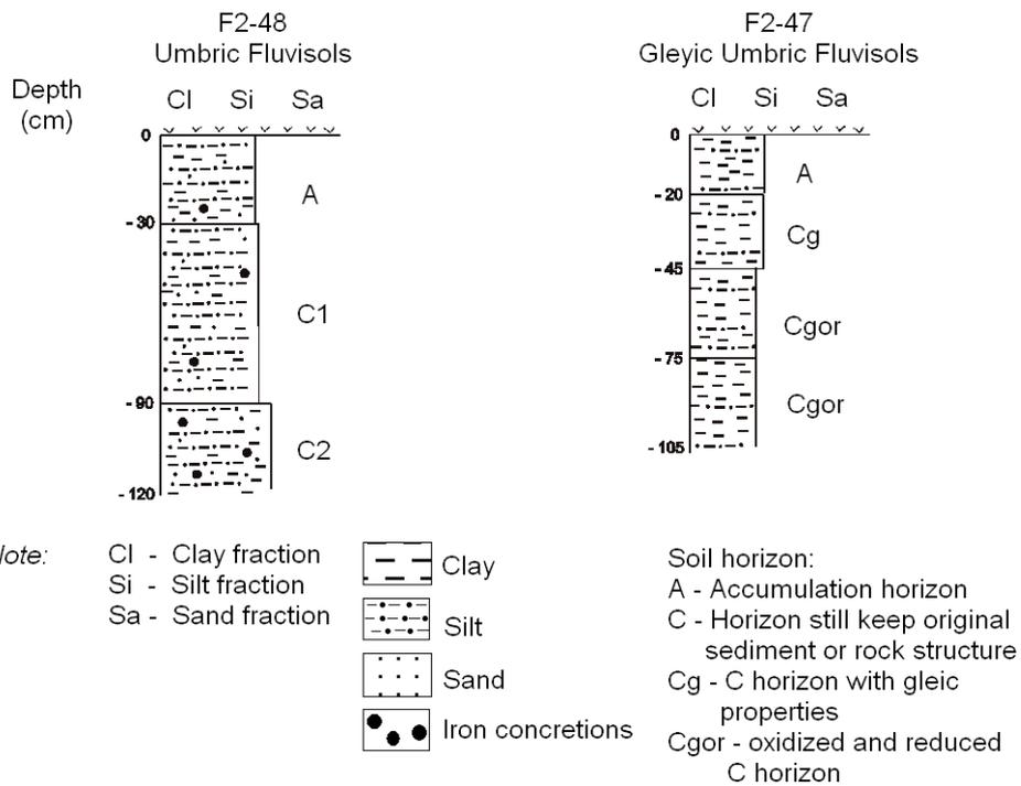
**Figure 3.14:** Catena F2-48 crosses the paleochannel. The soil samples are F2-47, -48.
