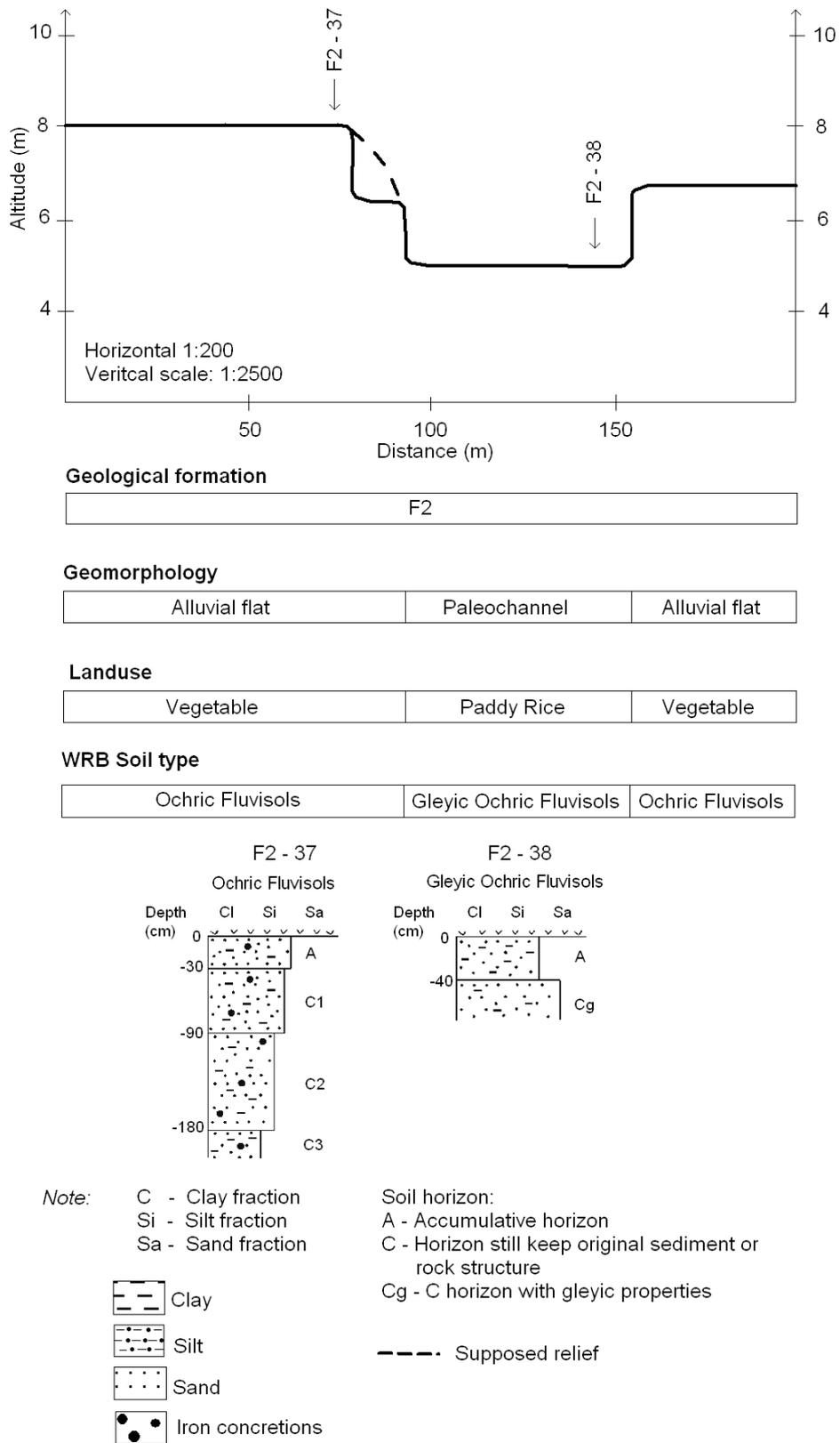
**Figure 3.15:** Catena F2-37 crosses the paleochannel. The soil samples are F2 -37, - 38.
