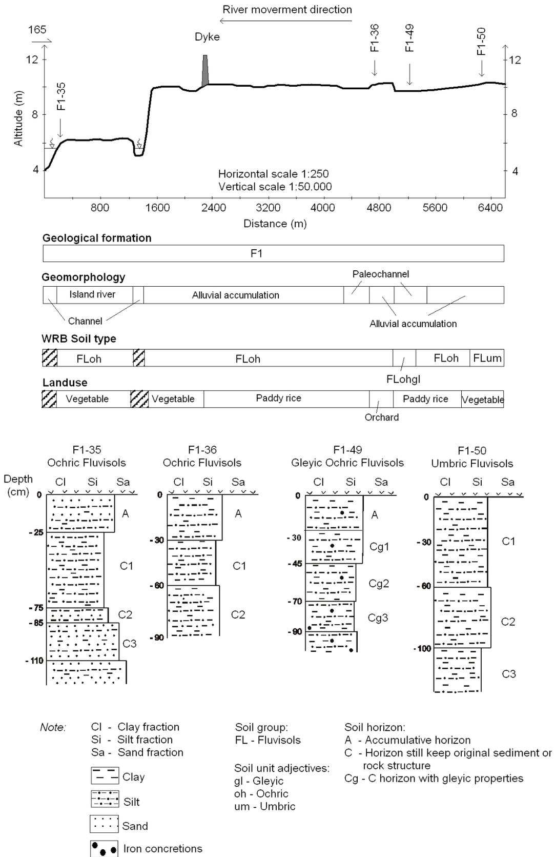
**Figure 3.13:** Catena F1 from the channel to alluvial accumulation. The samples are in F1 formation.
