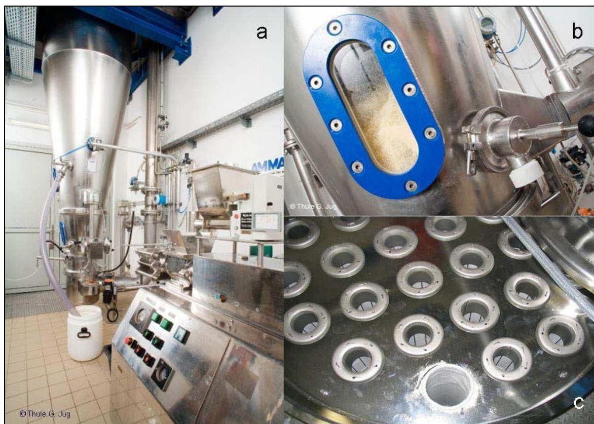
Figure 1 Photographs of the fluidised bed granulator at the Institute for Environmental Biotechnology, Department of Agrobiotechnology, IFA-Tulln, Austria, illustrating a. the lower part of the granulator next to a twin screw extruder, b. a detailed picture of the conical product chamber showing fluidised particles and the sampling device, and c. the filter unit located in the upper part of the granulator.
