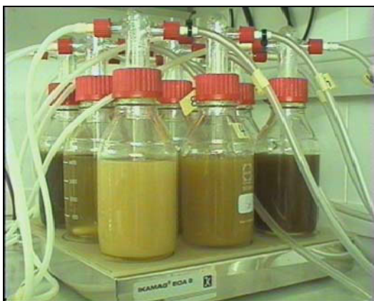
Figure 10 Experimental setup of the Modified Sturm Test according to OECD Guideline 301 B.
