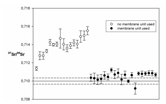
Fig. 15 Effect of USN and membrane for particle separation on measured <sup>87</sup>Sr/<sup>86</sup>Sr isotope ratio
