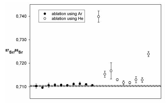
Fig. 17 Effect of use of Ar and He as ablation gases for hydroxyl-apatite spiked with NIST SRM 987 SrCO<sub>3</sub>
