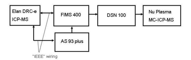
Fig. 10 Experimental arrangement of automated on-line FI Sr/matrix separation
