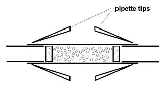
Fig. 7 Leak proof Sr/matrix separation column design
