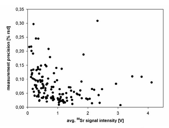
Fig. 22 Precision of single ablation events plotted versus average <sup>88</sup>Sr signal intensities during ablation
