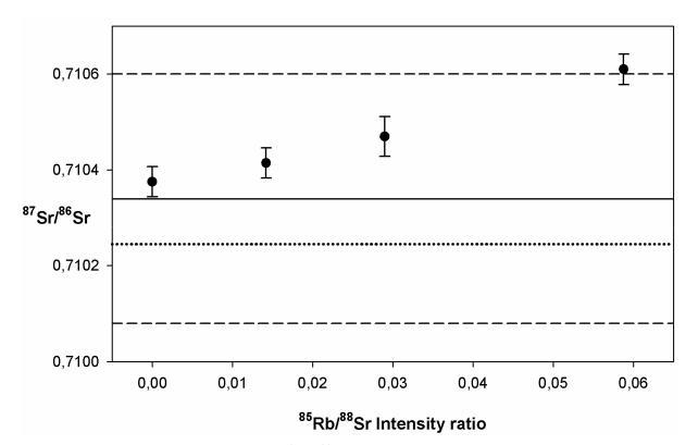
**Fig. 2** Linear increase of corrected <sup>87</sup>Sr/<sup>86</sup>Sr isotope ratio with increasing Rb concentrations; solid black line corresponds to certified isotope ratio, dashed black lines correspond to certified uncertainties, dotted black line corresponds to "accepted" value of 0.710245
