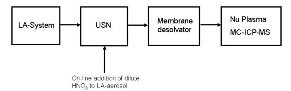
Fig. 13 LA-MC-ICPMS setup employing a USN and membrane desolvator for particle separation
