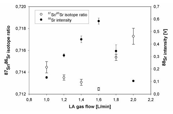
Fig. 18 Influence of LA gas flow on signal intensity and final measurement result
