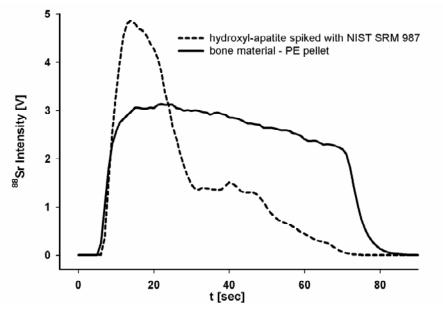
Fig. 19 Laser ablation signal profiles of reference targets
