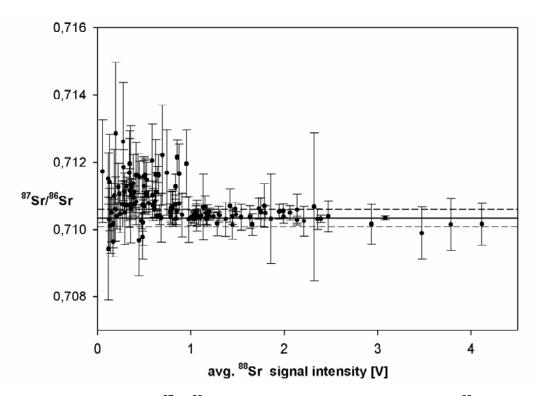
**Fig. 21** Measured <sup>87</sup>Sr/<sup>86</sup>Sr isotope ratio plotted versus average <sup>88</sup>Sr signal intensities during ablation; straight lines correspond to certified value
