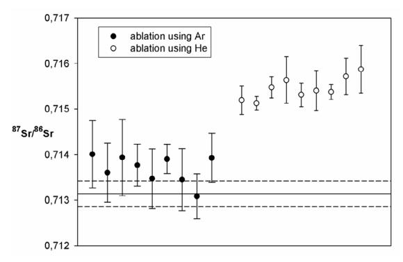
Fig. 16 Effect of use of Ar and He as ablation gases for NIST 1400 bone ash - PE pellet
