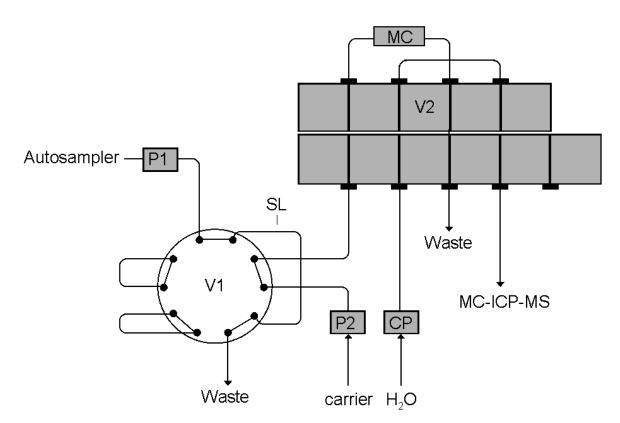
Fig. 11 Automated FI manifold for on-line Sr/matrix separation
