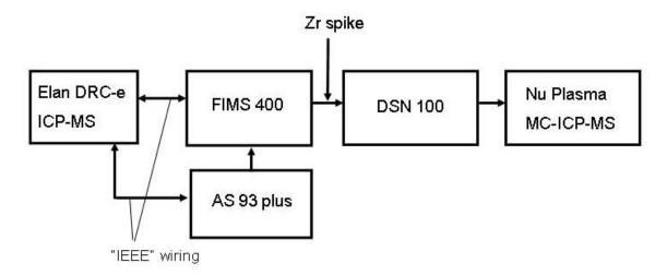
Fig. 12 On-line Addition of Zr spike for Sr isotope analysis
