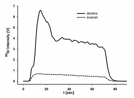
Fig. 20 Laser ablation signal profiles of archaeological tooth samples
