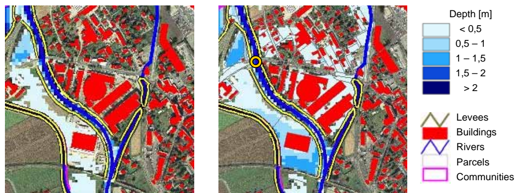
Figure 4.11: Inundations without (l.) and with jammed bridges. The exposed B 65 Bridge is marked (r.)
