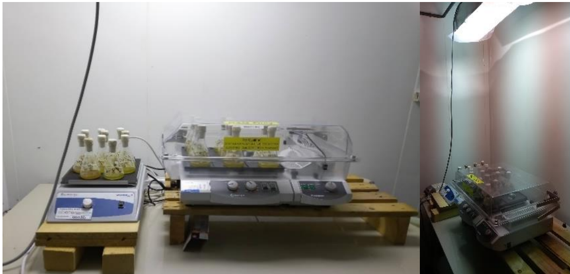
Figure 16: Setup temperature experiment. Left: regular shaker at RT (left side) and Titramax 1000 at 25°C (right side); Right: setup with halogen-metal vapor lamp.
