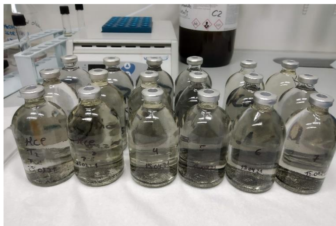
Figure 7. Glass bottles (120 mL) used for the microcosm experiment with PTFE/butyl rubber septa and crimp caps to ensure anaerobic conditions.
