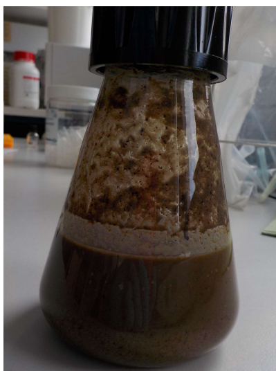
Figure 3: Enzymatic hydrolysis of OMSW in a conical flask.
