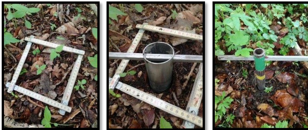
Figure 5. Demonstration of sampling procedure, from left to right: 15x15 cm frame for litter sampling, 5 cm metal core marked at 10 cm length for soil sampling, and 2 cm metal core marked at 10 cm length for root sampling.
