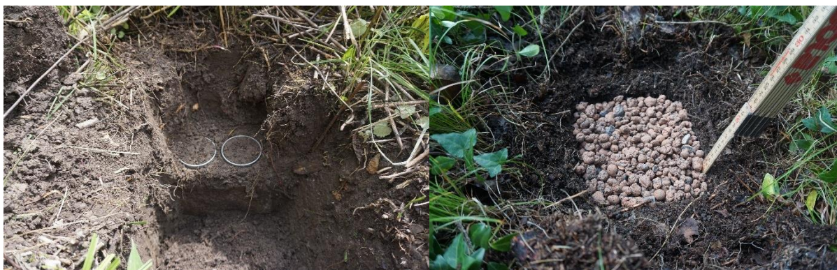
Figure 7: Sampling method for obtaining soil samples from Fluvisols (left) and Rendzic Leptosols (right)
