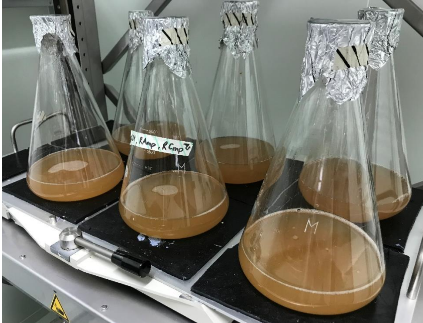
Figure 17: Fermentation of cytochrome cz in 2-L shaking flasks.
