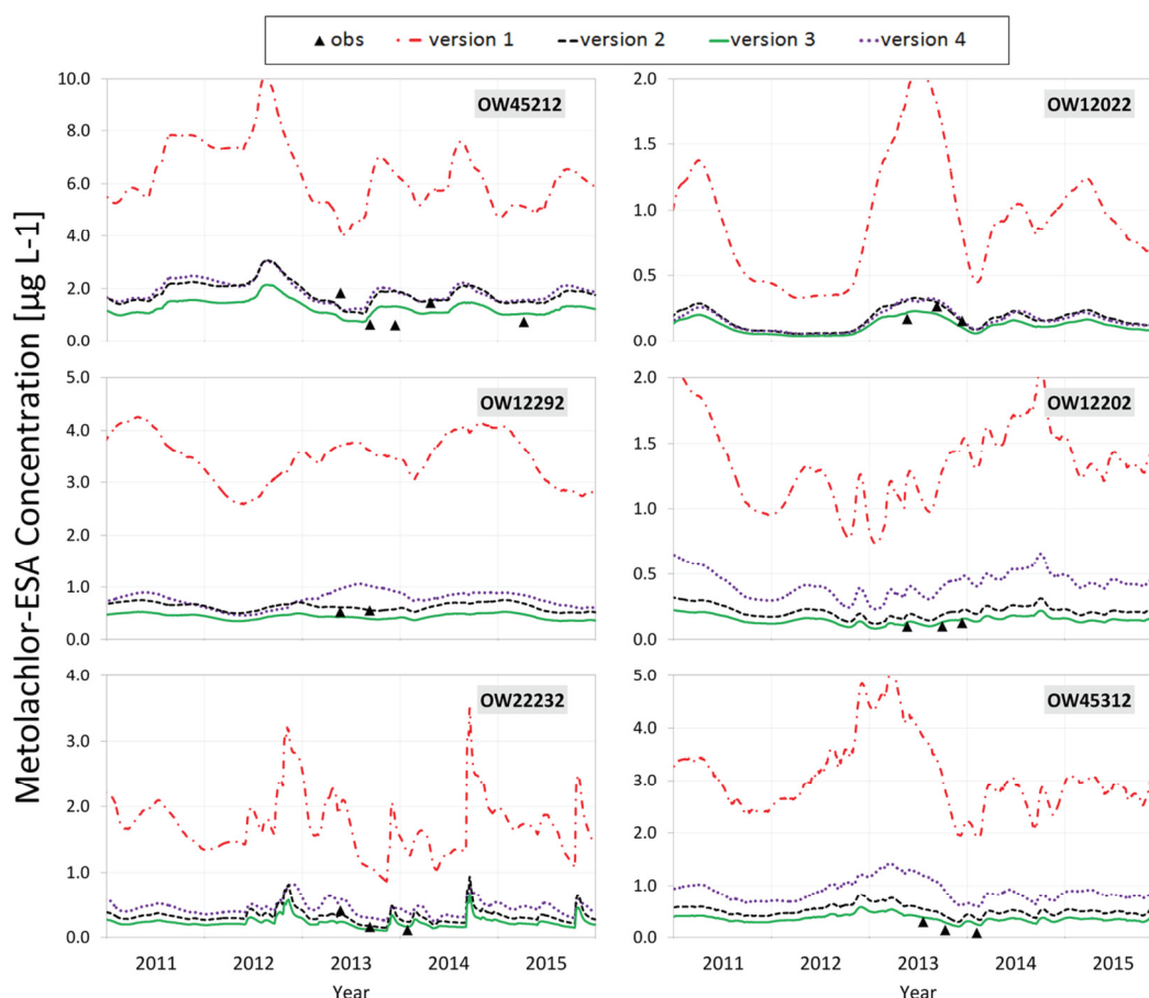
Fig. 5. Metolachlor ethane sulfonic acid (MESA) groundwater concentration time series as the available discrete measurements at monitoring wells OW45212, OW12292, OW22232, OW12022, OW12202, and OW45312 and simulated using no site-specific information (Version 1), uniformly distributed parameters derived from site-specific calibration (Version 2), a 30% reduction in applied volume of S-metolachlor to quantify input dosage uncertainty (Version 3), and soil-specific fate parameters applied to 750% of the agricultural area following the results of the laboratory analysis for the investigated surface soil types and the 30% dose reduction from Version 3 (Version 4).
