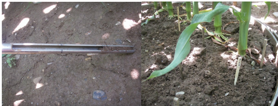
Figure 4.6: Soil sampling with a stainless steel auger; each borehole was marked
