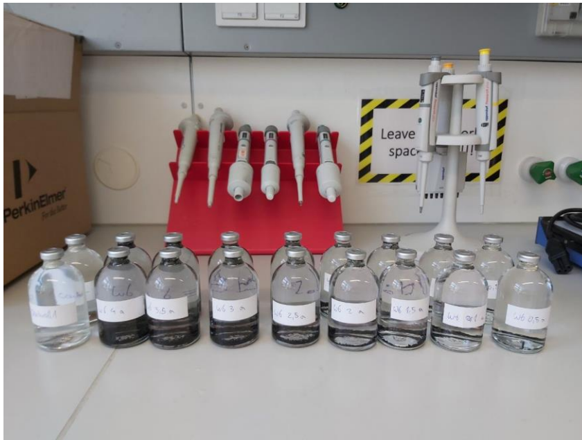
Figure 9: 120 ml serum bottles with crimp caps and PTFE septa after filling.
