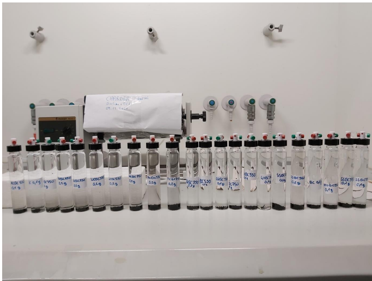
Figure 8: 60 ml headspace vials with mininert caps and varied adsorbent dose (100, 200 mg).
