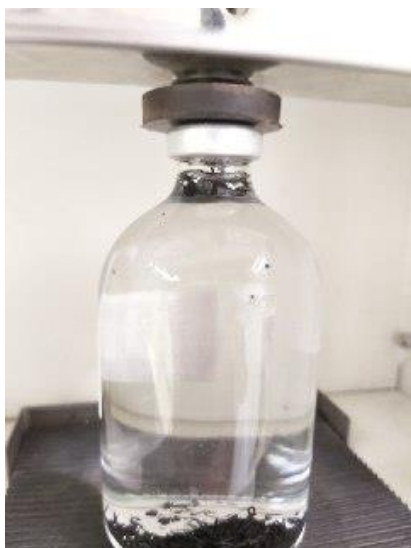
Figure 25: Biochar particles floating on top after 96 h.
