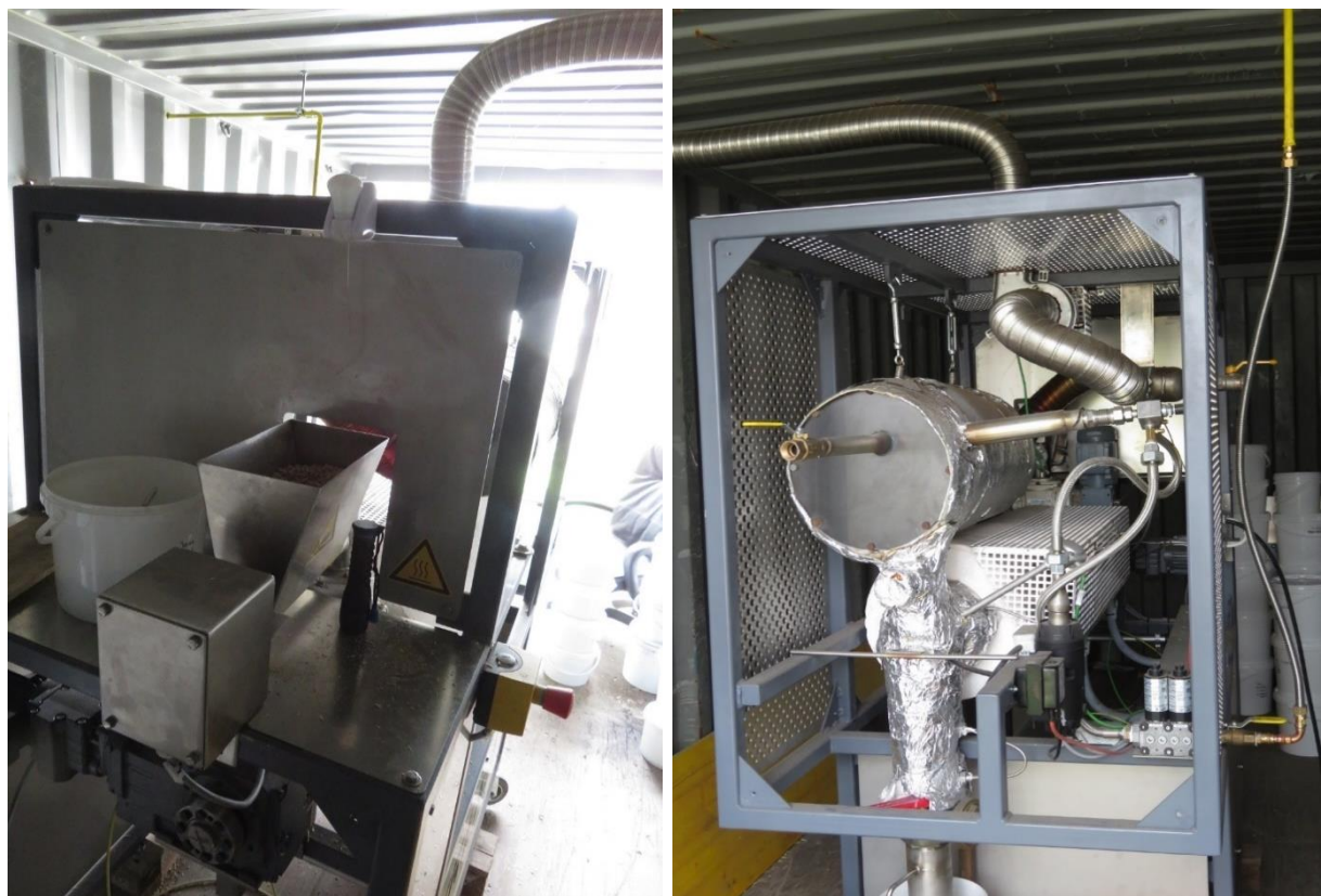
Figure 6: PYREKA feeder and screw reactor, discharge container and burning chamber (personal archives, 2020)
