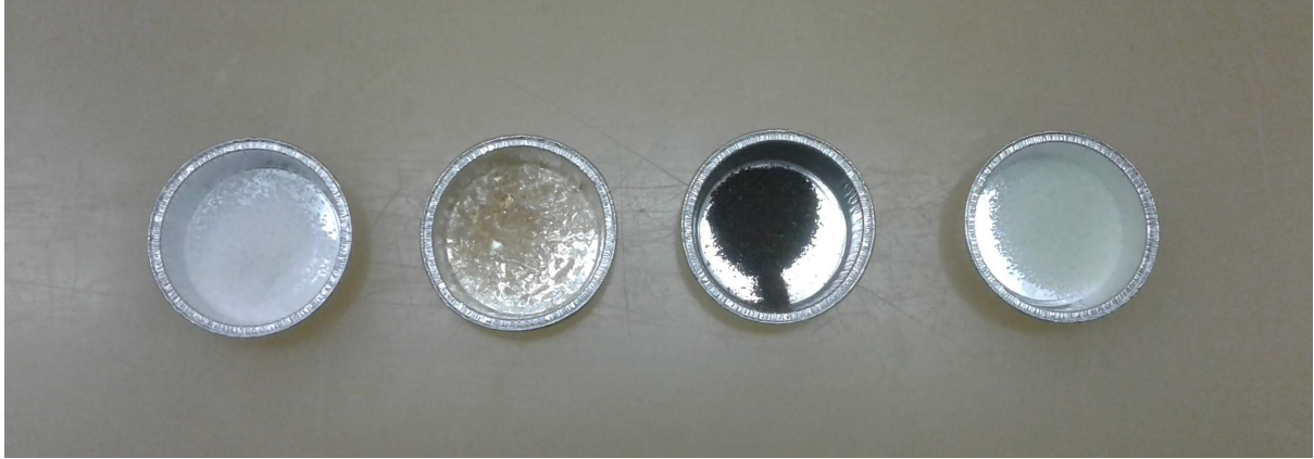
Figure 1: Tested hydrogels from left to right: Stockosorb, Cellulose, Lignin and fine grained Polyter.
