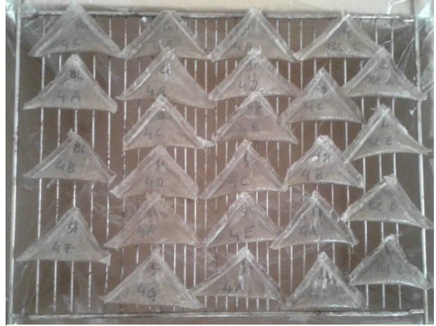
Figure 3: Triangular mesh bags containing sand and hydrogel during the dripping process
