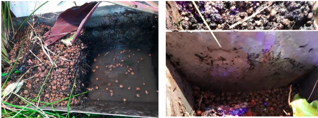
Fig. 5.6: Removal of the clogged substrate at the end of phase I
