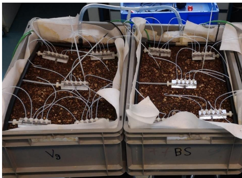
Figure 3. Multi-drip outlet irrigation system of two experimental plots connected with T-splitter (left: vegetated, right: non-vegetated).
