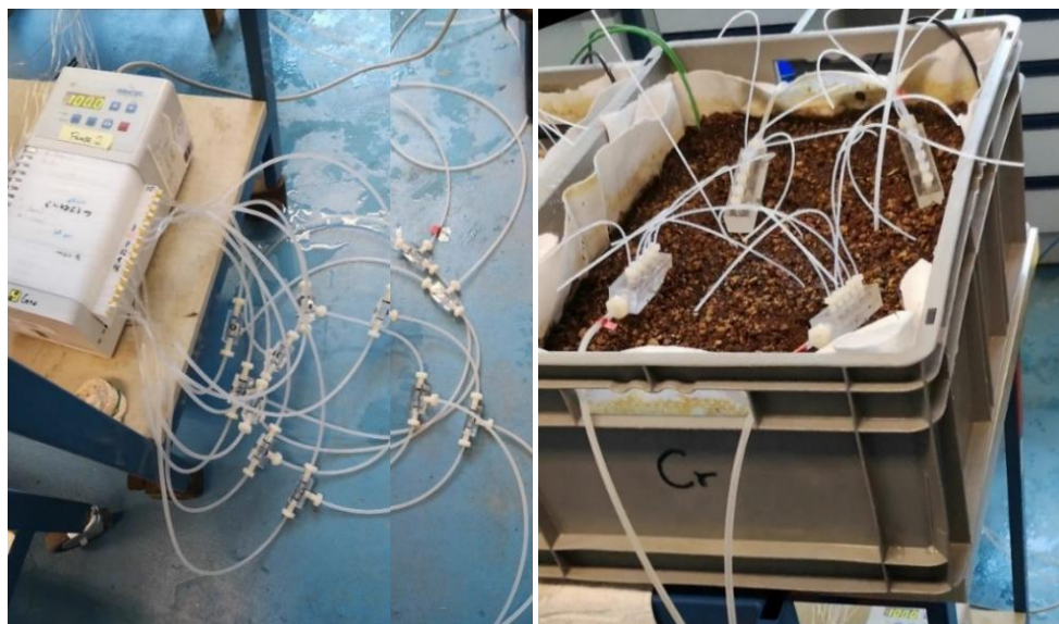
Figure 4. Irrigation system in the control plot (Left: Two-level parallel connection of capillary pipes from the peristaltic pump, Right: Multi-drip outlets delivering the water near surface)
