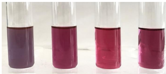
Figure 23 Colour of colloidal GNPs solutions (from left to right: pH = 3, pH = 4, pH = 5, pH = 6)
