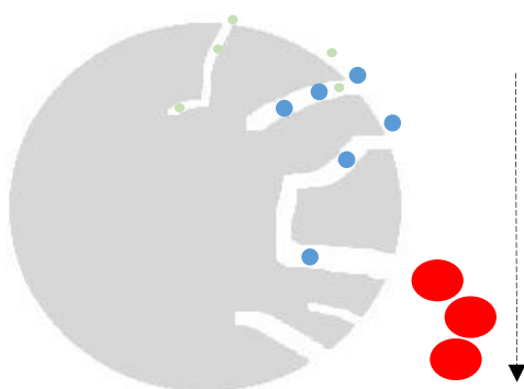
Figure 8: Principle of Size exclusion chromatography. Exclusion of larger particles of the internal pores (own illustration)
