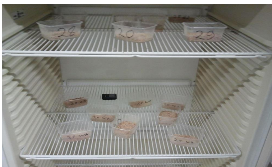
Figure 3.1 One of nine incubators used, with boxes containing larvae and feed: Boxes were placed randomly in incubators and a data logger (testo 174 T ® , black device in picture) was used to monitor temperature and relative humidity.
