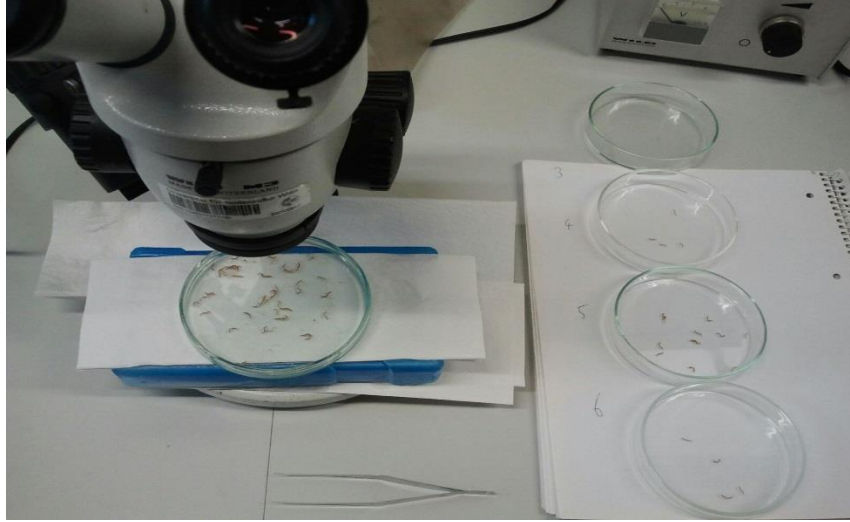
Figure 3.3 Measurement of head capsule width with WILD Heerbrugg microscope with an ocular micrometer 10x21, calibrated with an object micrometer. Larvae were separated on ice (blue) according to their instar (Table 3.3).
