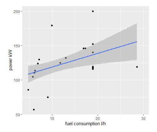
Figure 32 - Regression line of loader's power and fuel
