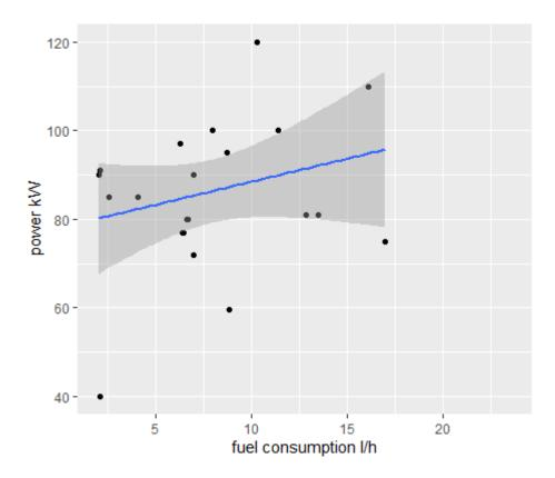
Figure 26 - Regression line of tractor's power (kW) and fuel (I/PMH)
