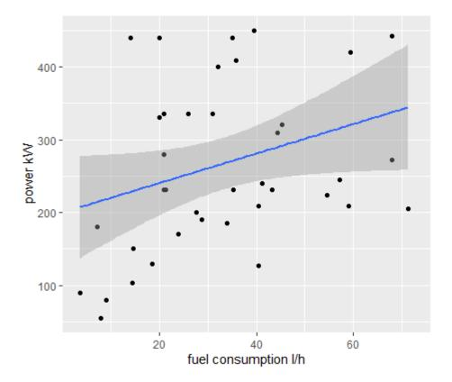
Figure 35 - Regression line of chipper's power and fuel
