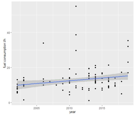
Figure 22 - Forwarder's fuel consumption over time (year weighted by machine's power)
