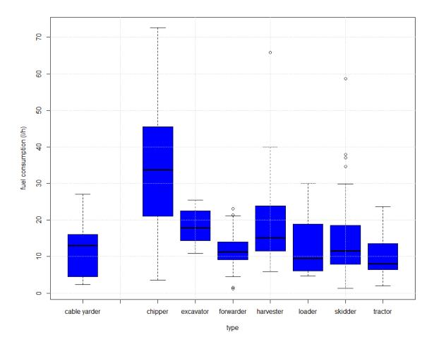
Figure 7 - Diesel driven machine's fuel consumption in I/PMH
