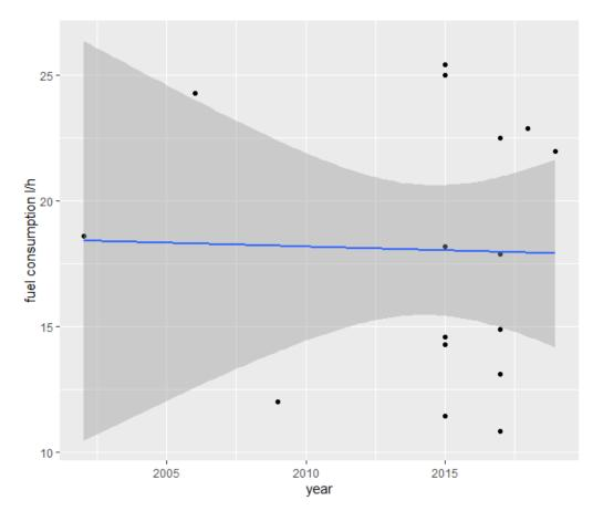
Figure 31 - Excavator's fuel consumption over time (year weighted by machine's power)
