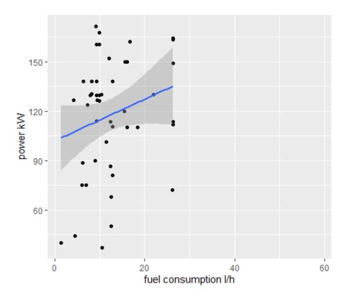
Figure 23 - Regression line of skidder's power (kW) and fuel (I/PMH)
