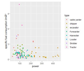
Figure 10 - Diesel driven machine's specific consumption per cubic meter over power
