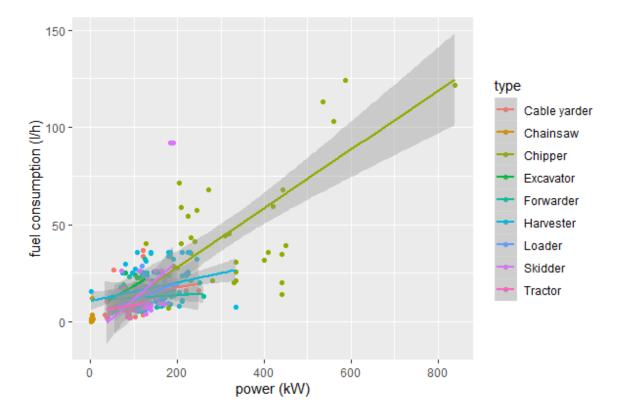
Figure 9 - Diesel driven machine's power and fuel regression
