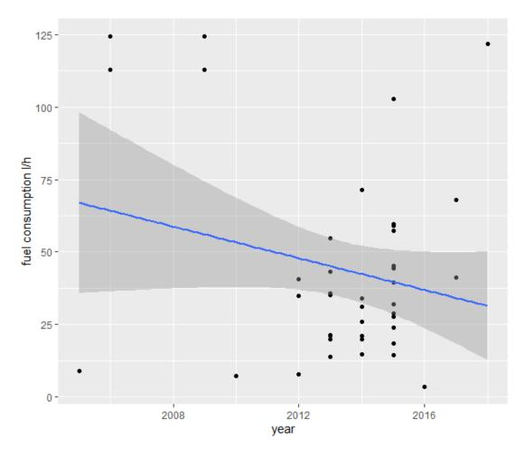
Figure 37 - Chipper's fuel consumption over time (year weighted by machine's power)
