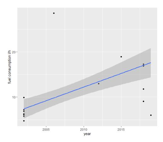
Figure 34 - Loader's fuel consumption (I/PMH) over time (year weighted by machine's power)
