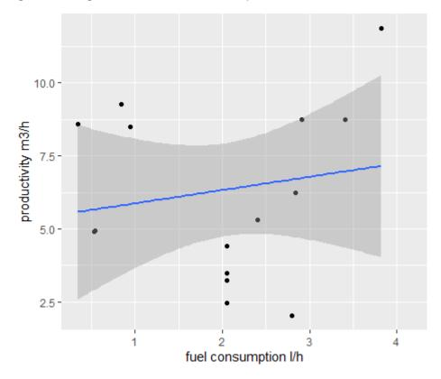
Figure 12 - Regression line of chainsaw's productivity and fuel consumption
