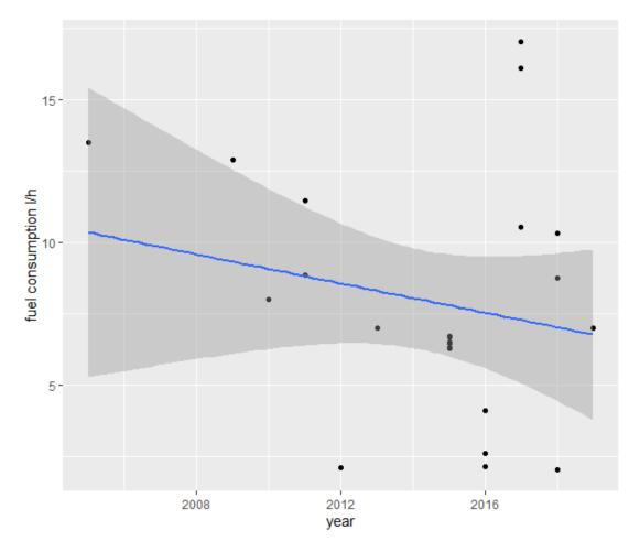
Figure 28 - Tractor's fuel consumption over time (year weighted by machine power)
