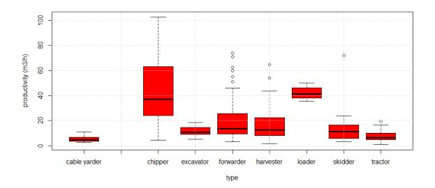
Figure 6 - Diesel driven machines' productivity in m<sup>3</sup>/PMH
