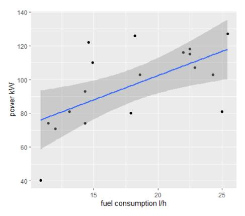
Figure 29 - Regression line of excavator's power and fuel
