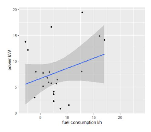
Figure 11 - Regression line of chainsaw's power and fuel
