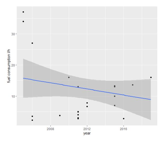
Figure 19 - Cable yarders fuel consumption over time (year weighted by machine's power)
