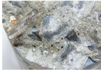
Fig. 24 Specimens with ASR signs
