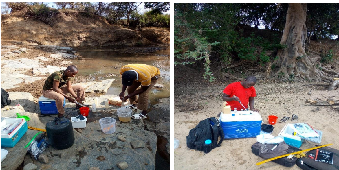
Photo 3: Preparation of water samples for nutrient, DOC, Chlorophyll a and TSS analysis
