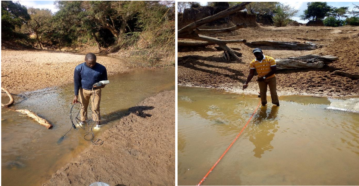
Photo 2: In-situ measurement of water quality variables and discharge
