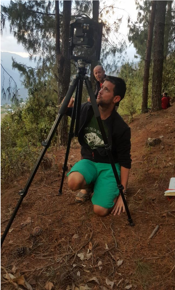
Image A9: Fisheye lens camera on the self-levelling mount and tripod
