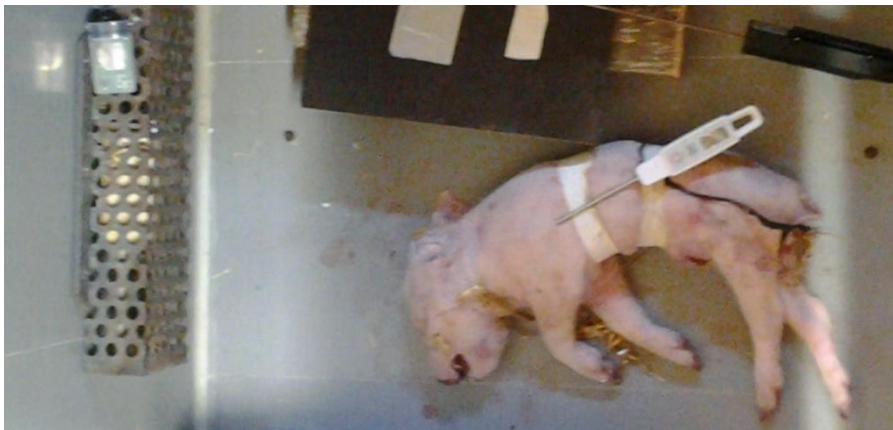
Figure 9. Subcutaneous temperature measurements in a dead piglet and concurrent measurement of the ambient air temperature.
