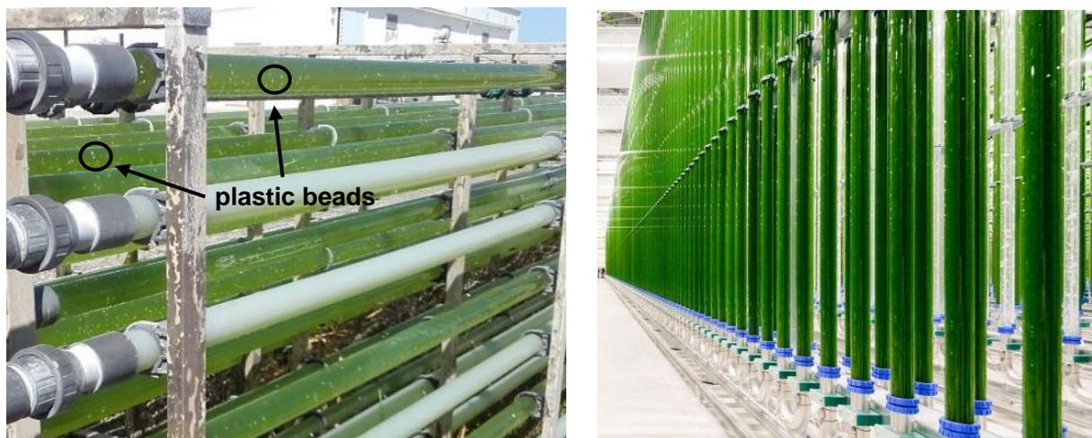
**Figure 2: Left: Horizontal tubular photobioreactor with plastic beads. Reactor was built in the course of the project “Integrated Sustainable Algae” in Olhao, Portugal. © Meixner. Right: Large scale vertical tubular photobioreactors, eparella GmbH production plant. (ecoduna, 2018)**
