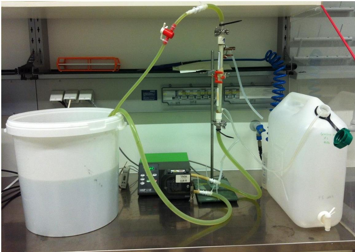
**Figure 13: Setup of cross-flow filtration unit for biomass harvest.**
