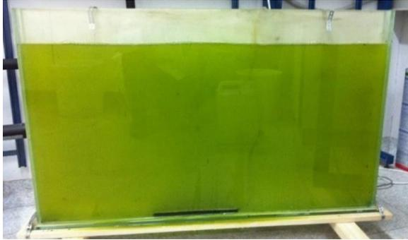
**Figure 3: Laboratory-scale flat plate reactor (20 L working volume).**
