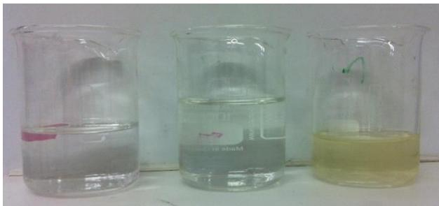
Figure 31: Colour comparison. From left to right: RO-H<sub>2</sub>O, process water after cross-flow filtration, process water after centrifugation. Pictures are from second harvest.
