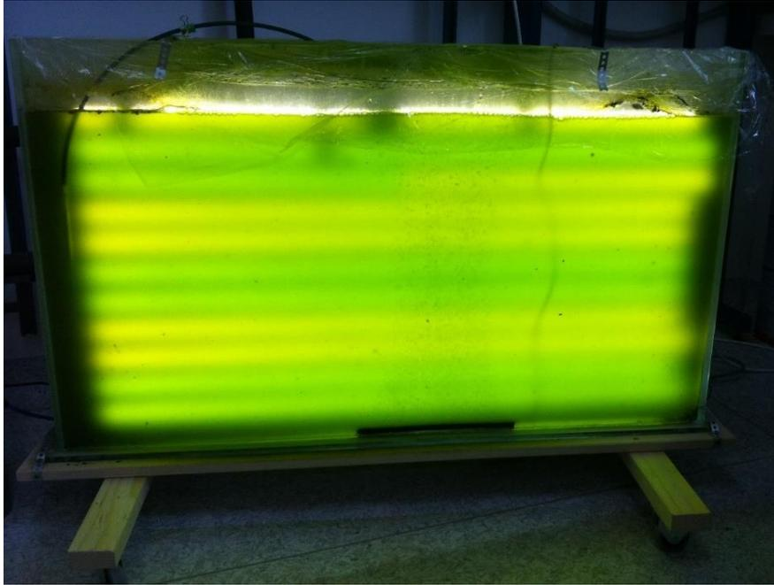
**Figure 12: Flat plate reactor filled up to maximum working volume of 20 L, all lights on and CO<sub>2</sub> supply installed.**
