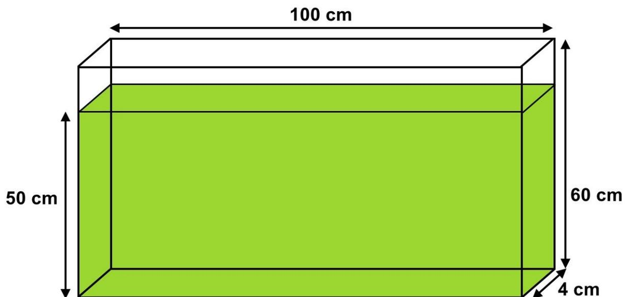
Figure 11: Illustration of flat plate reactor.
