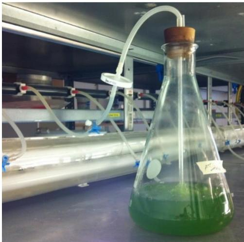
Figure 6: Setup of 2-L flask aerated with ambient air.
