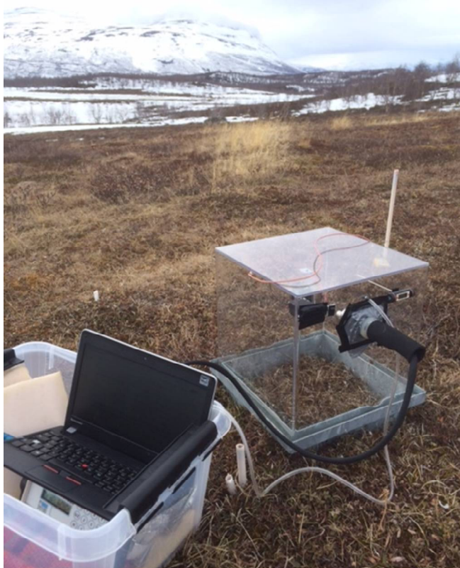
Figure 3: Transparent gas flux measurement chamber for NEE measurement on metal frame connected to EGM-4 and laptop in early spring (Foto: Anders Michelsen)
