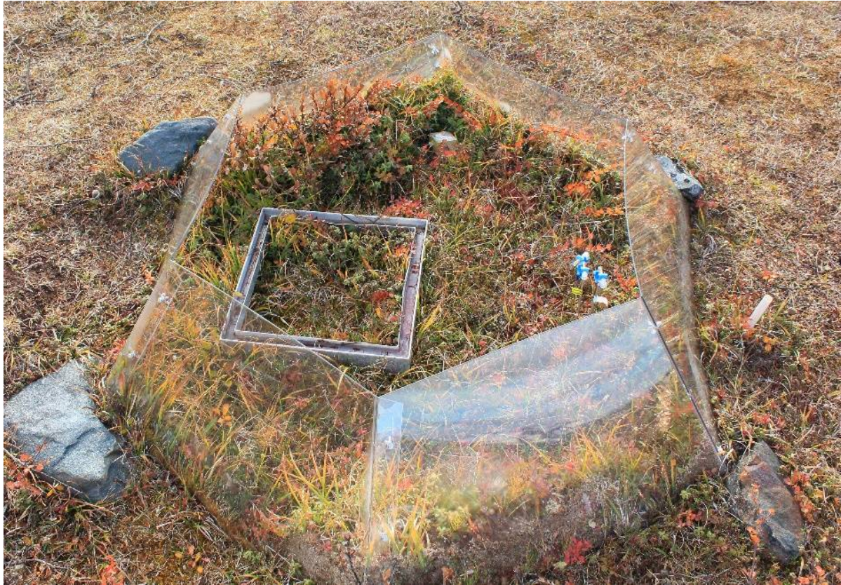
Figure 2: Warming treatment plot with OTC and 33 x 33 cm metal frame for CO 2 flux measurements. (Photo: Anne Schäfer)
