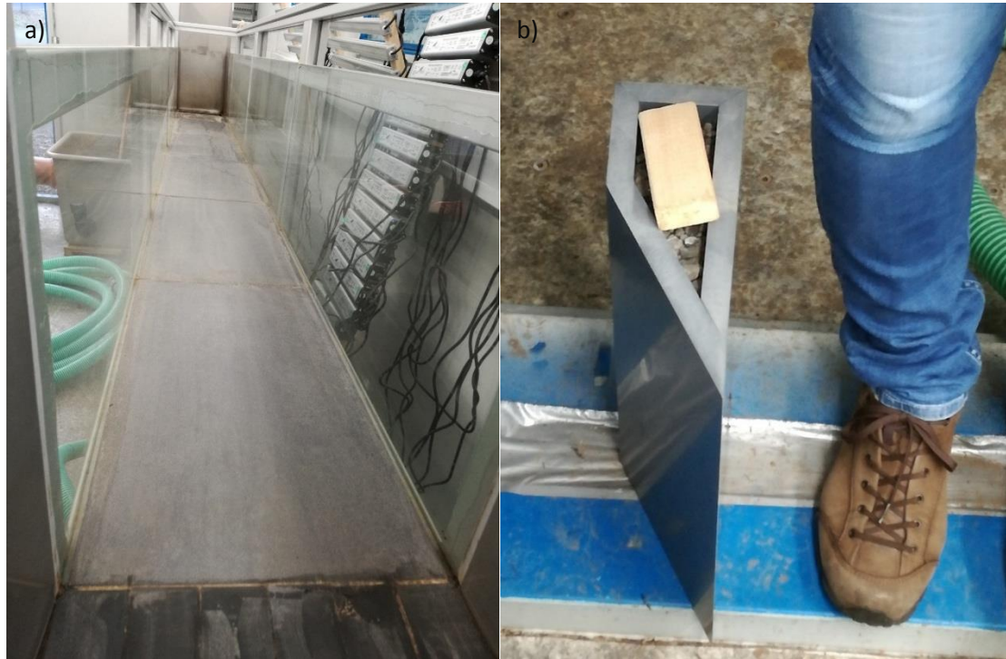
Figure 3: a) on the left, the flow channel with the artificial substrate (black tiles) is shown. b) On the right, one of the current obstacles, which will be placed on both sites at three transects, is shown.
