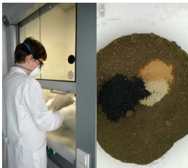
Figure 3. Soil spiking: Mixing soil with lead oxide (left figure), Addition of soil amendments: biochar, gravel sludge and iron oxides (from left to right) (right figure)
