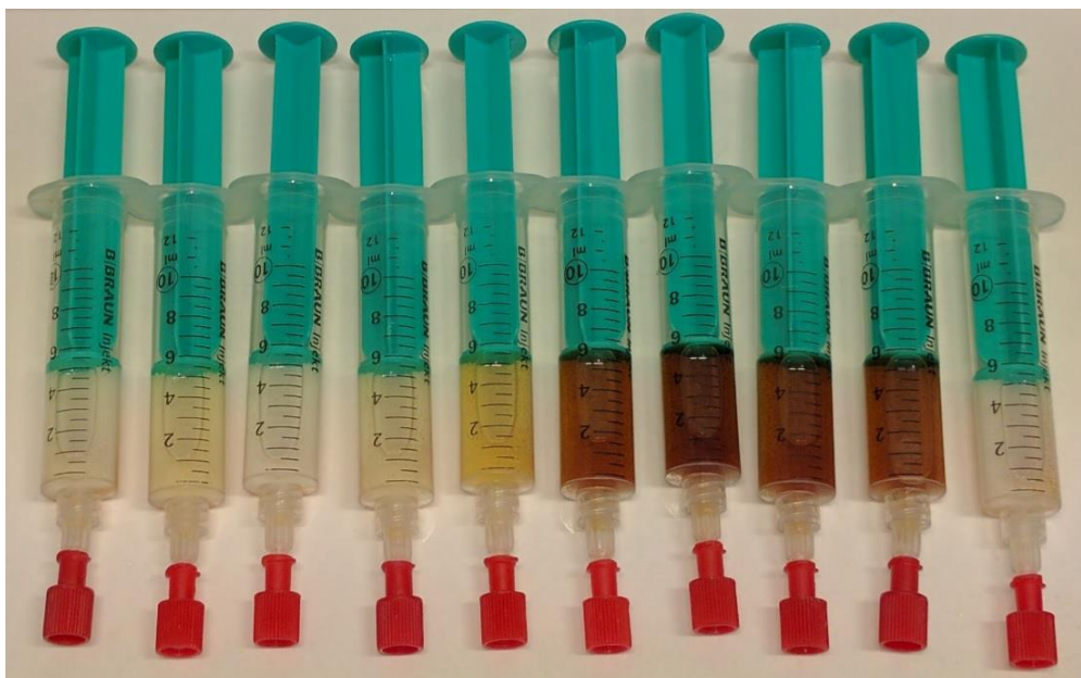
Figure 17: Resin assisted extraction; micro scale approach by (SUMERSKII ET AL., 2015). Samples from the 1 M experiment; left (0 minutes) to right (360 minutes or bubbling loss). Dark color indicates solubilization of lignin fragments with increasing reaction time.
