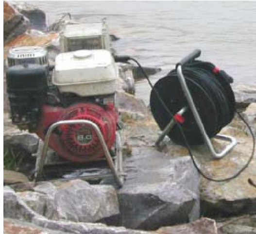
Figure 11: Stationary electrofishing unit (Wiesner 2003)
