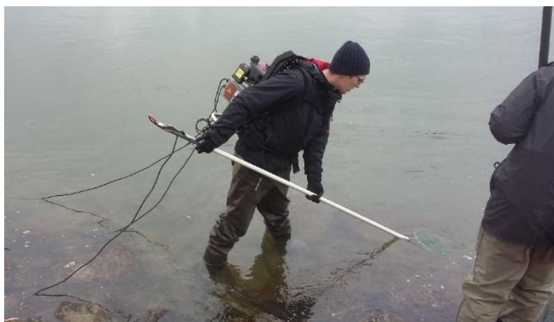
Figure 10: Sampling with a portable electrofishing unit
