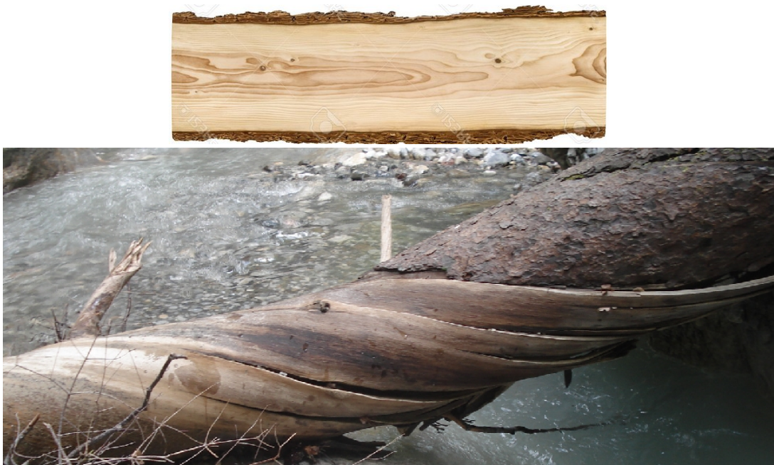
Figure 4: The pattern on sawed wood is not influenced by spiral grain. Thus, the board (top) could well originate from a log with spiral grain (bottom).
