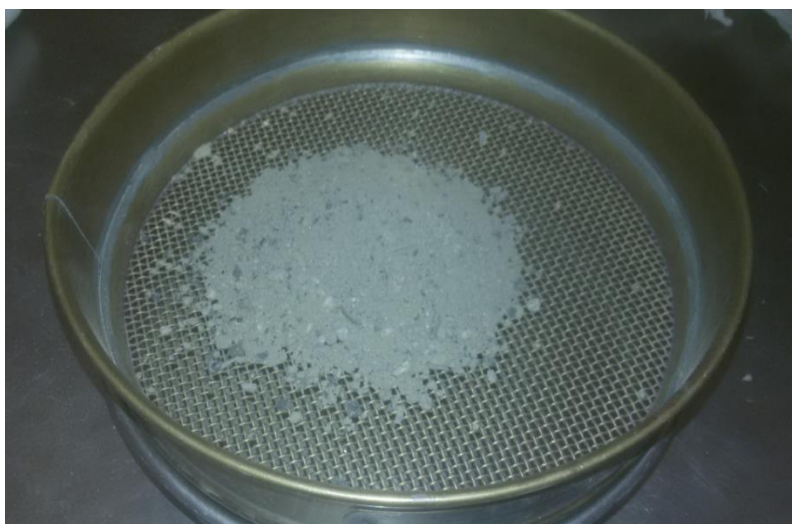
Figure 8: Air dried soil was sieved with a 2.00 mm soil sieve.
