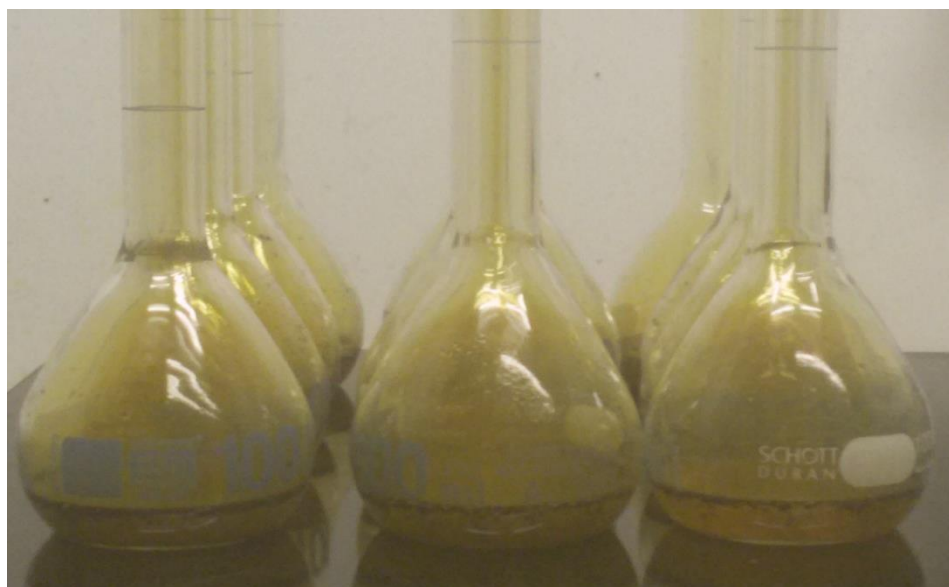
Figure 10: Last step of sequential extraction- aqua regia digestion of soil samples on the heating plate. The yellow vapour origins from nitrous gases, which were driven out.
