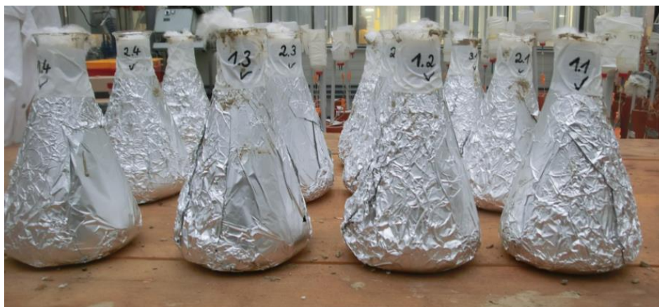
Figure 6: Soil incubation experiment with amendments in Erlenmeyer flasks 1.0 l Erlenmeyer flasks were covered with aluminium foil and closed with cotton plug.
