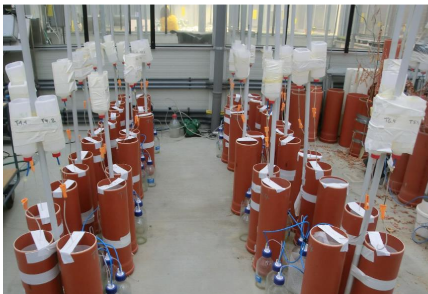
Figure 5: Two rows with 20 lysimeter each, which resulted in 40 randomly placed lysimeters.
