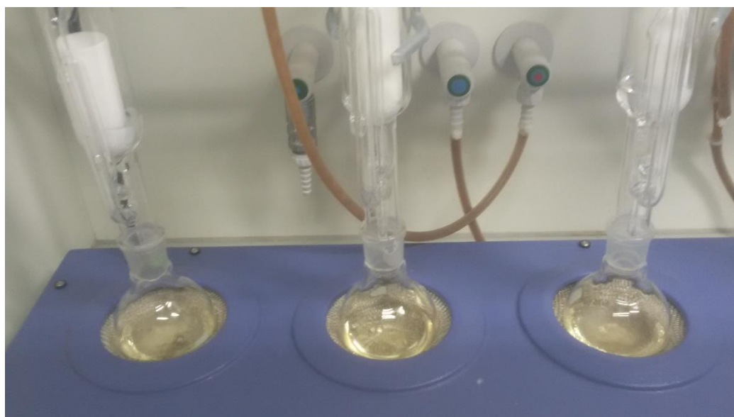
Figure 9: Soxhlet apparatus for the extraction of polycyclic aromatic hydrocarbons from soil.
