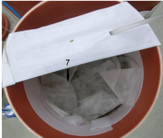
Figure 3: Water permeable fleece (7) to homogenize the water distribution over the soil surface.
