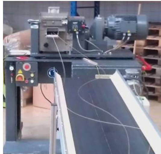
Figure 23 Left extruder Collin ZK25 with two parallel polymer strands, left Cutter Primo 100 with curvy polymer strands
