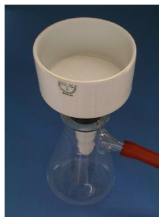
Figure 14 Büchner funnel with conical flask, Source [37]
