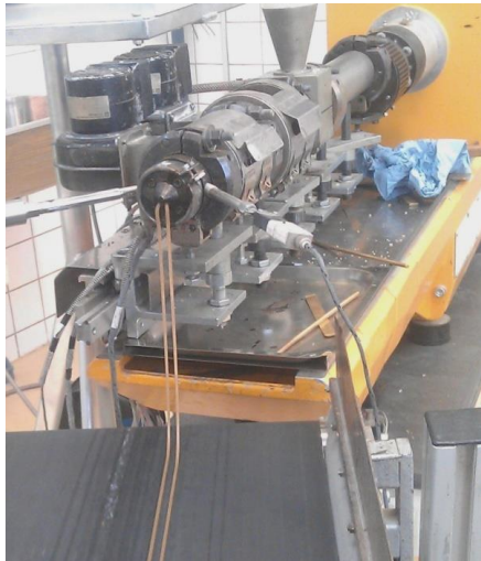
Figure 23 Left extruder Collin ZK25 with two parallel polymer strands, left Cutter Primo 100 with curvy polymer strands
