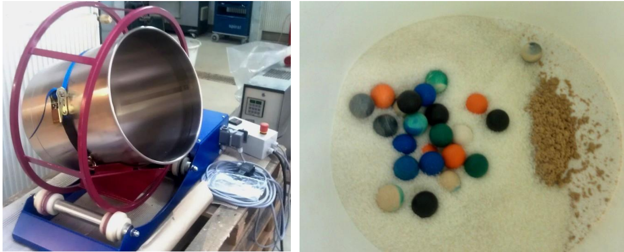
Figure 21 left picture mixing unit, right picture mixing balls with PLA and fibre sample
