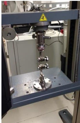
Figure 24 descriptive build up Tensile test
