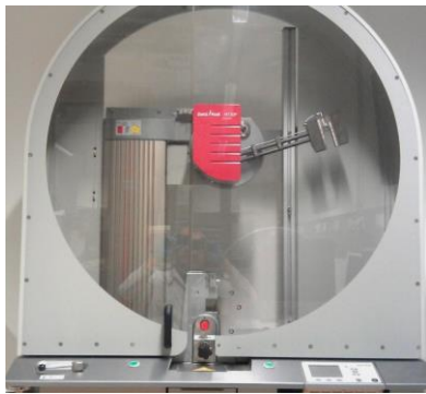
Figure 27 Zwick/Roell HIT50P impact strength testing machine
