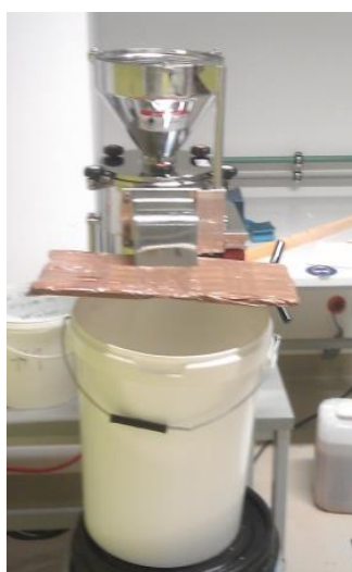
Figure 12 Microfibrillation of lignocellulose fibres with Masuko Ultrafine Grinder MKCA6-2J
