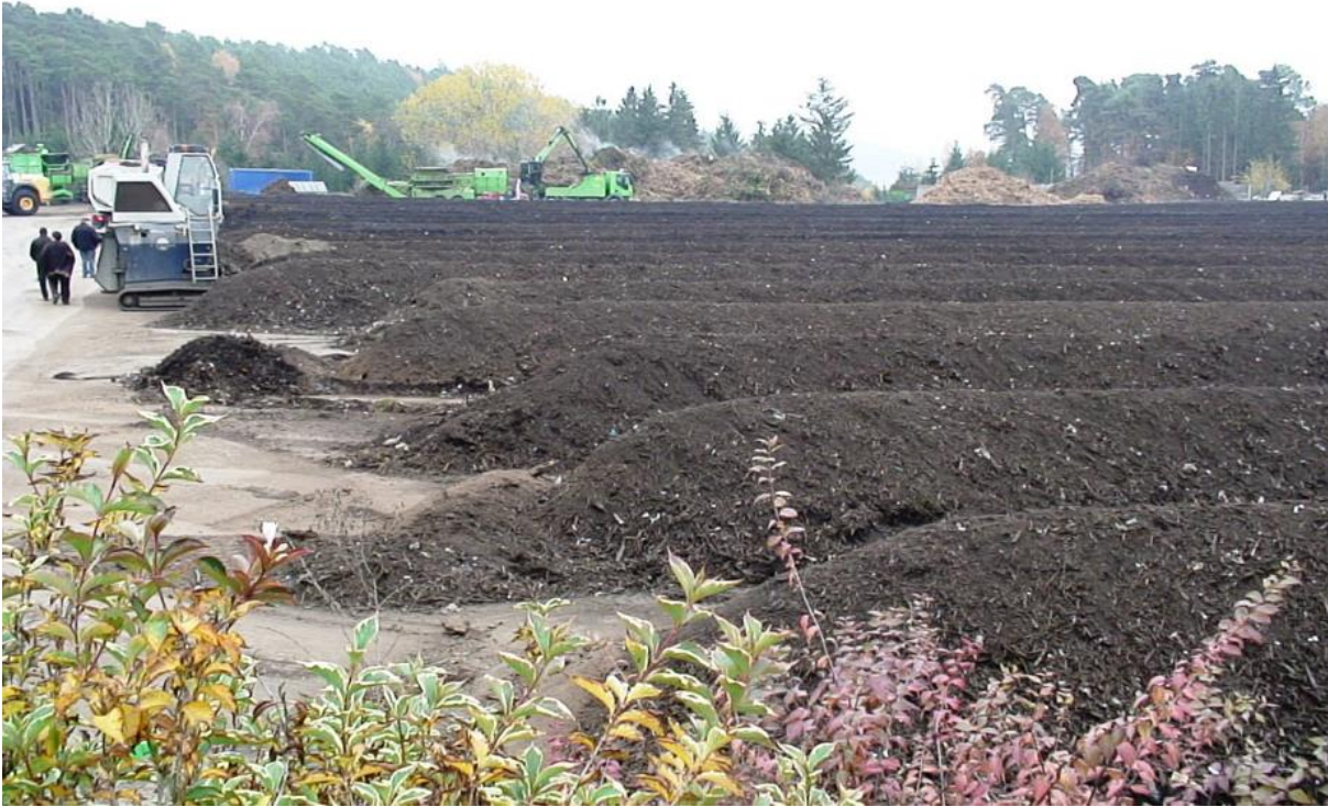
Figure 17: Example of open windrow composting, aerated piles (Binner, 2008)
