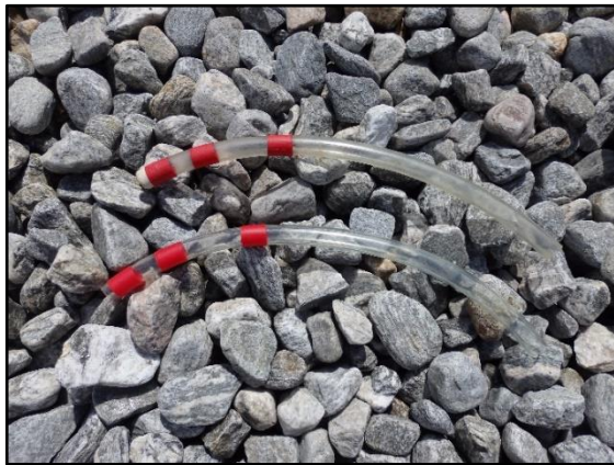
Figure 18: Plastic hoses to measure number and size of shelters.
