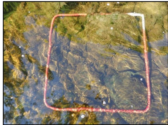
Figure 19: Steel frame ( 0.50 \times 0.50 \text{ m} ) to measure the shelter availability in a defined area ( 0.25 \text{ m}^2 ).
