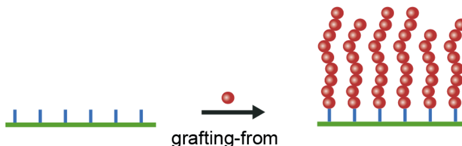
Figure 11: Scheme of a grafting-from polymerization on a modified surface (green and blue figure), yielding a higher brush (red chains) density than with the grafting-to method.
