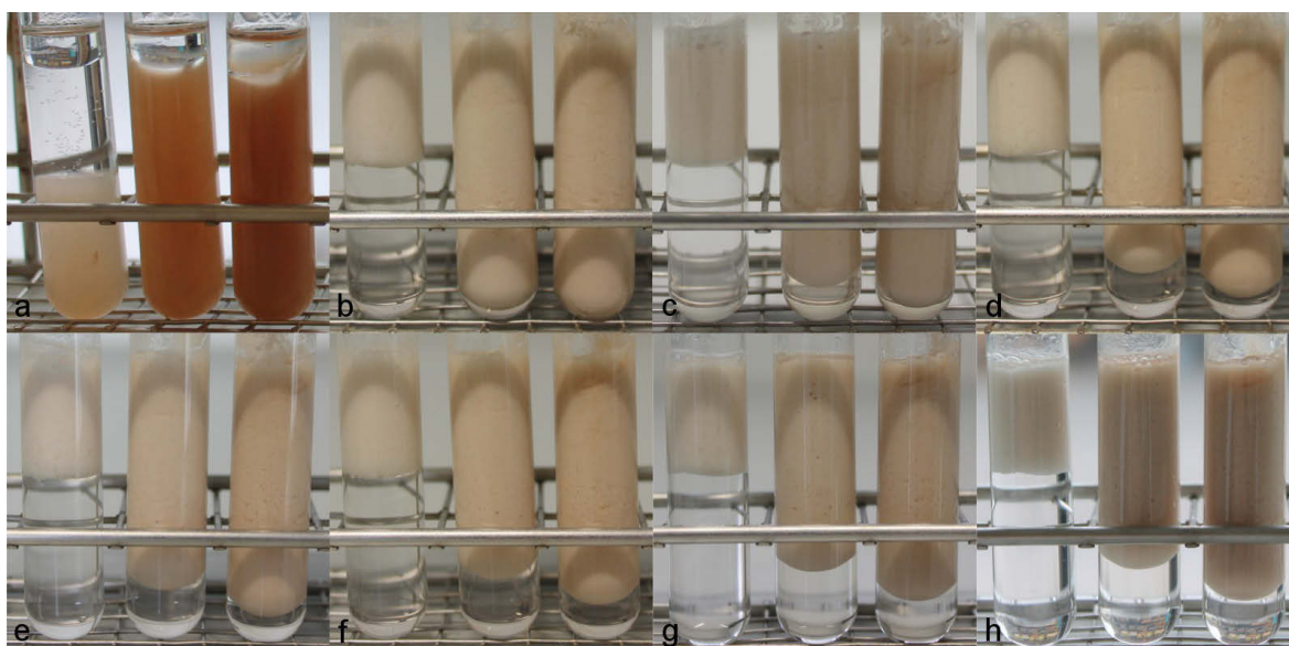
Fig. 5: Emulsions stabilised by MFLC before mixing(a), after mixing(b), after one(c), three(d), four(e) hours, after one(f), eight(g) and twelve(h) days. Concentrations are 0.1, 0.5 and 0.7% from left to right in each picture.
