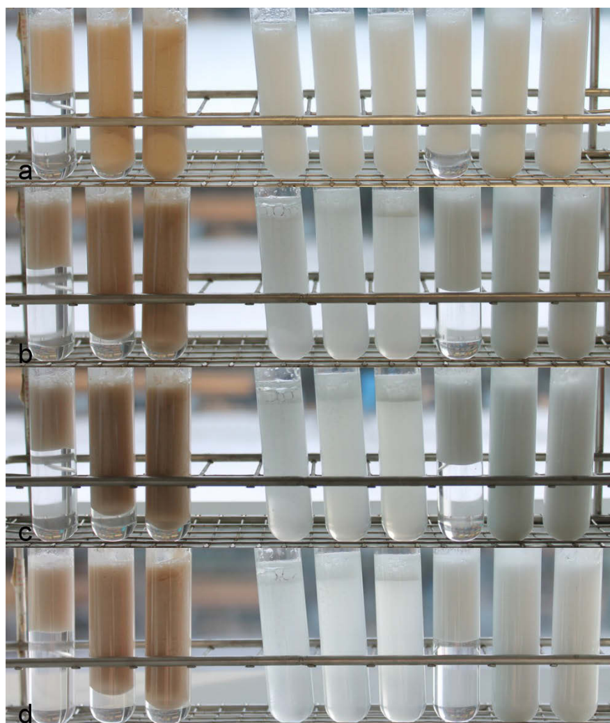
Fig. 4: Water-styrene emulsions after mixing (a), after one(b), three(c) and four(d) hours. From left to right: MFLC, CNC and MFC with concentrations of 0.1, 0.5 and 0.7% (w/w) each.
