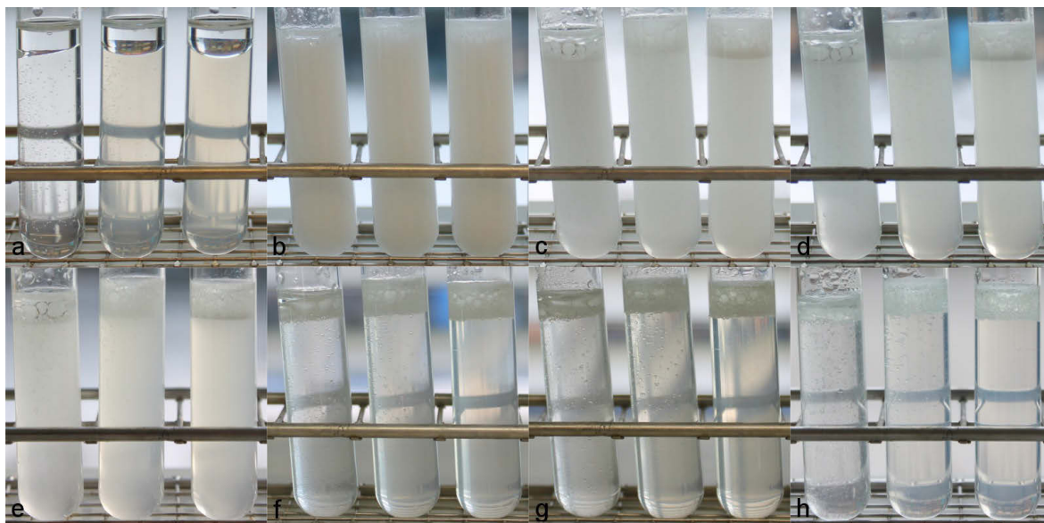
Fig. 6: Emulsions stabilised by CNC before mixing(a), after mixing(b), after one(c), three(d), four(e) hours, after one(f), eight(g) and twelve(h) days. Concentrations are 0.1, 0.5 and 0.7% from left to right in each picture.
