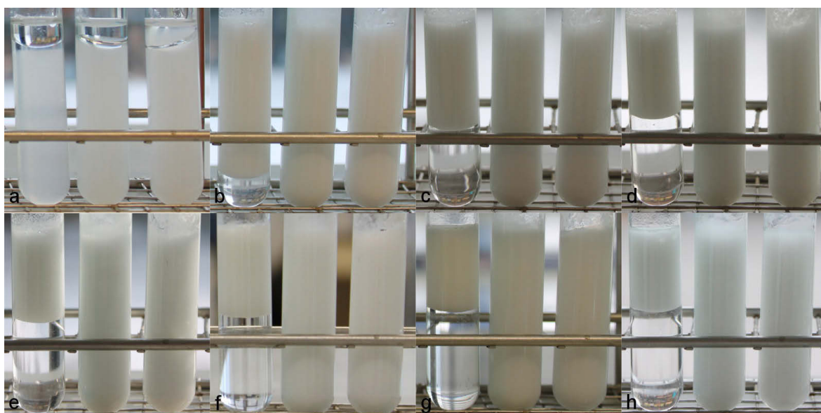
Fig. 7: Emulsions stabilised by MFC before mixing(a), after mixing(b), after one(c), three(d), four(e) hours, after one(f), eight(g) and twelve(h) days. Concentrations are 0.1, 0.5 and 0.7% from left to right in each picture.
