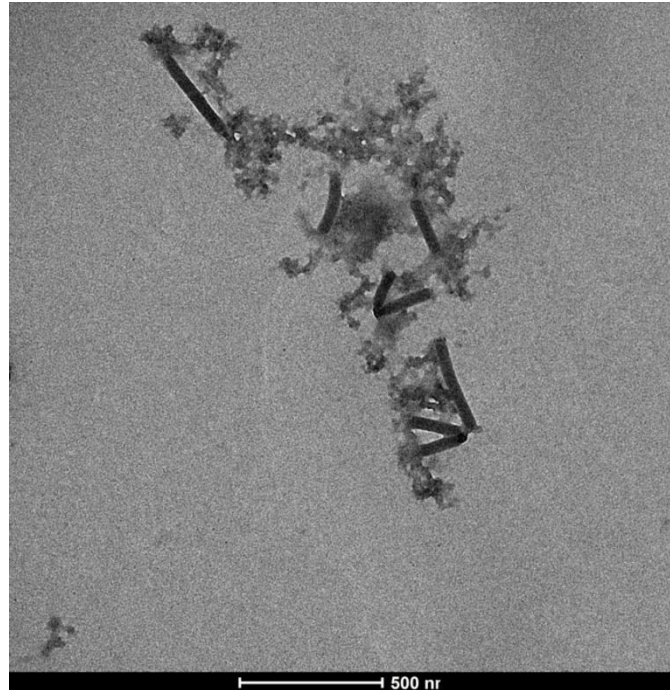
Figure 4-20: Image of TEM measurement of (Sf9 CD64 \Sigma + M1) at 19000 x magnification.
