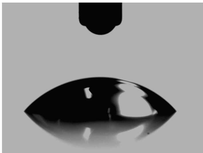
FIGURE E.10: Contact angle measurement of water on COP + SiO 2 + GLYMO + Diaminopropane (1:80)
