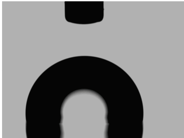
FIGURE E.1: Contact angle measurement of water on COP
