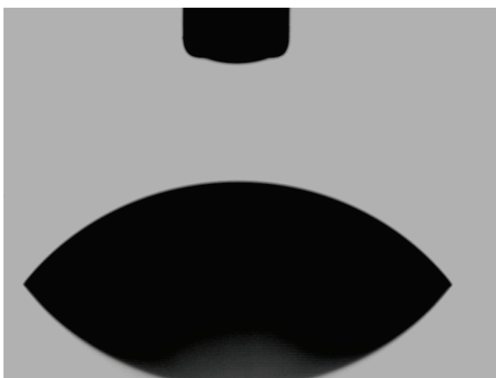
FIGURE E.9: Contact angle measurement of water on COP + SiO 2 + GLYMO + Ethylenediamine (1:80)
