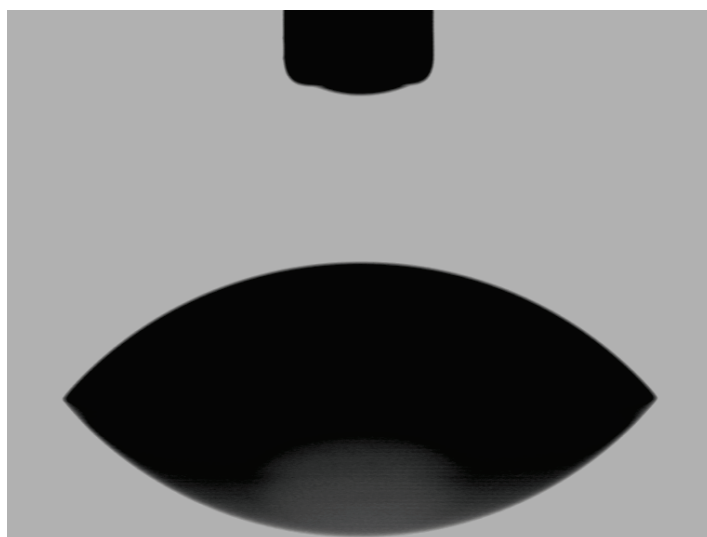
FIGURE E.7: Contact angle measurement of water on COP + GLYMO
