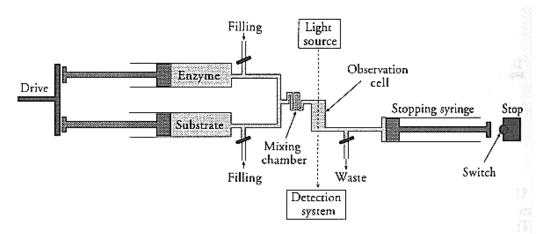
Figure 3-6: Scheme of stopped-flow apparatus with convential mixing mode
