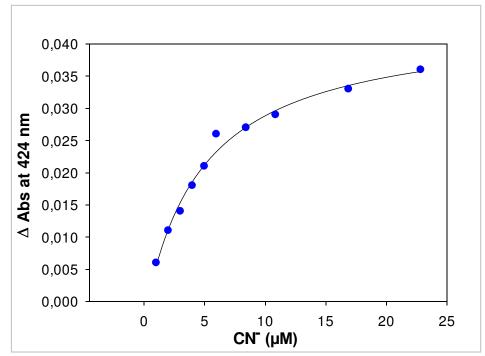
Figure 4-18: Absorbance differences at 424 nm plotted against increasing sodium cyanide concentrations
