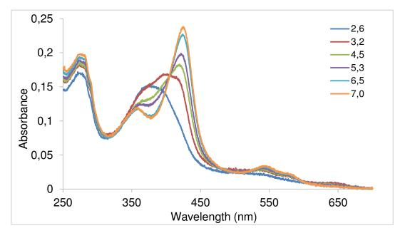
Figure 4-8: UV/vis spectra of AnHTP at different pH values in the acidic pH range
