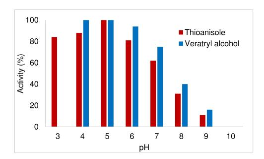
Figure 4-11: Sulfoxidation and alcohol oxidation activity of AnHTP in % over a pH range of 3 to 10. 100 % are corresponding to 32.7 U/mg and 3.0 U/mg, respectively.
