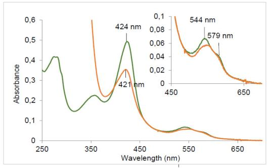
Figure 4-10: Non-reduced (green) and reduced (orange) UV/vis spectrum of *An*HTP
