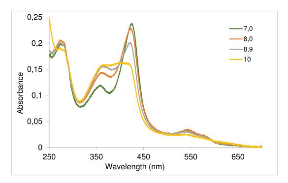
Figure 4-9: UV/vis spectra of AnHTP at different pH values in the basic pH range
