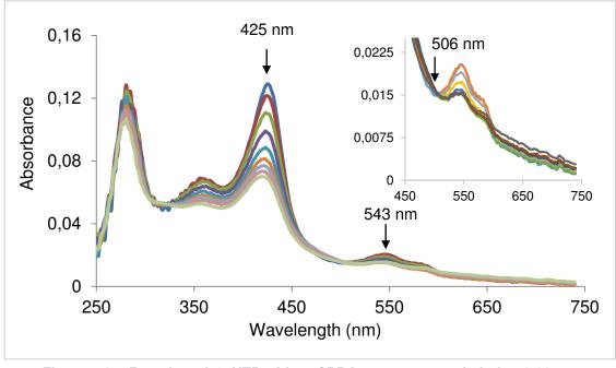
Figure 4-25: Reaction of *An*HTP with *m*-CPBA, spectra recorded after 0.005 s, 0.066 s, 0.136 s, 0.317 s, 0.561 s, 0.947 s, 1.56 s, 3.53 s, 6.51 s. The arrows show the decrease of absorbance with time at a specific wavelength.
