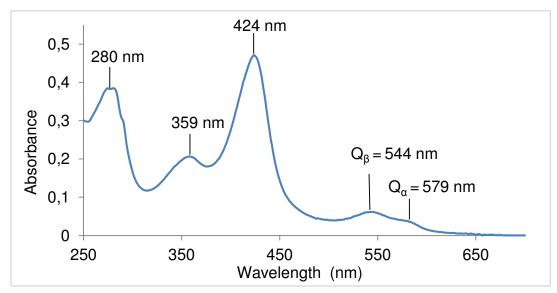
Figure 4-5: UV/vis spectrum of purified AnHTP
