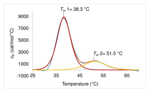
Figure 4-23: Differential scanning calorimetry thermogram of AnHTP
