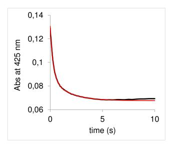
Figure 4-26: Double exponential fit (red) of change of absorbance at 425 nm over time
