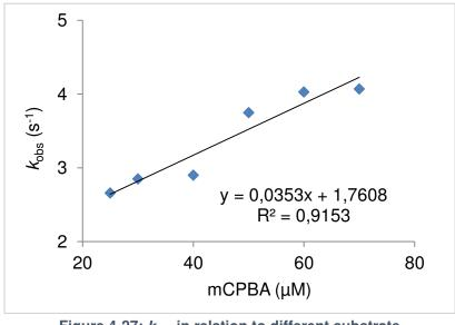
Figure 4-27:  $k_{obs}$  in relation to different substrate concentrations,  $k_{app}$  can be obtained from the slope of the linear fit
